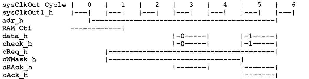
0. The cReq\_h pins are always idle in the system clock cycle immediately before the beginning of an external transaction. The adr\_h pins always change to their final value (with respect to a particular external transaction) at least one CPU cycle before the start of the transaction.
