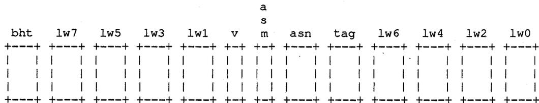
Bits within each field are arranged such that high-order bits are on the left. The serial chain shifts to the right.
