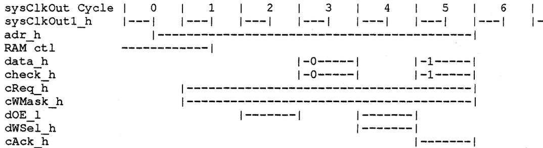
0. The cReq\_h pins are always idle in the system clock cycle immediately before the beginning of an external transaction. The adr\_h pins always change to their final value (with respect to a particular external transaction) at least one CPU cycle before the start of the transaction.
