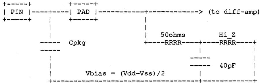
This is designed to approximate a 50ohm termination for the purpose of impedance matching for those systems (if any) which drive input clocks across long traces. Furthermore, the high impedance bias driver allows a clock source of arbitrary DC bias to be AC coupled to EV4. The peak-to-peak amplitude of the clock source must be between 0.6V and 3.0V as seen by EV4. Either a "square-wave" or a sinusoidal source may be used. Note that full-rail clocks may be driven by testers.
