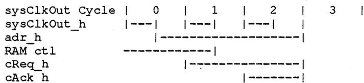
0. The cReq\_h pins are always idle in the system clock cycle immediately before the beginning of an external transaction. The adr\_h pins always change to their final value (with respect to a particular external transaction) at least one CPU cycle before the start of the transaction.
