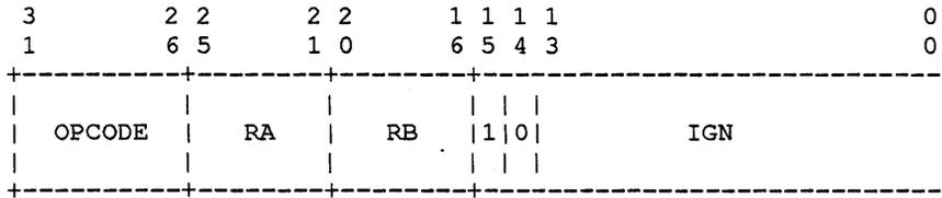
Note that bits[15..14] contain the branch prediction hint bits. EVx pushes the contents of the EXC\_ADDR register on the JSR prediction stack. Bit[15] must be set to pop the stack to avoid misalignment. The next address and PALmode bit are calculated as follows:
