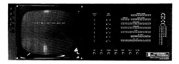
Figure 9. PDP-1/A CRT console.
