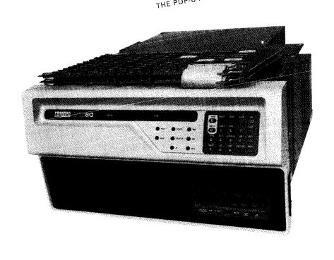
Figure 15. PDP-8/A processor.
