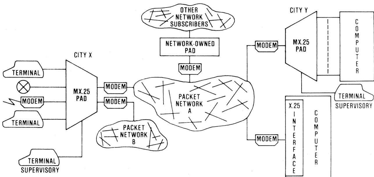
Figure 2. Typical Microplexer network application. If the unit is equipped with dual synchronous links, it can access more than one public data network.
