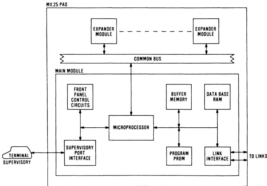
Figure 1. Main module functional block diagram. The main module and expander modules are linked via a common bus.
