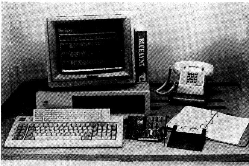
*The Techland Blue Lynx 5251 provides the IBM PC or PC XT with the capabilities of an IBM 5251 Model 12 display. With it, users can connect remotely to an IBM System/34, System/36, or System/38. The package consists of a half size expansion card, emulation software, a keyboard map, and documentation.*
