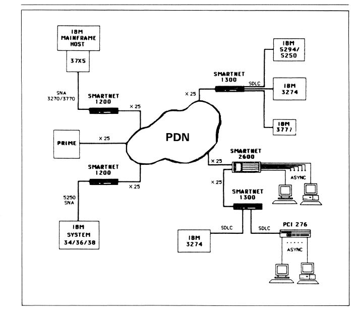
Figure 1. Shown above is a typical application using the SmartNet Series 1000 units and the SmartNet 276. Also in the network is the SmartNet 2600, a switching Packet Assembler/Disassembler (PAD) that provides asynchronous-to-X.25 protocol conversion.
