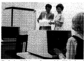
The Sanders 8100 is actually part of the 800 family and includes as standard, a 5 megabyte disk drive. Standard software is included to accommodate data entry/validation operations as well as operation as a remote batch terminal using the IBM 2780 discipline.
