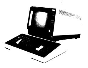
The Raytheon PTS/1200 Distributed Processing System provides support for up to 32 display stations and/or printers. Both 9-inch (shown here) and 15-inch displays can be used with the system.
