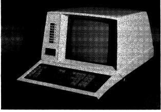
A PTS 100 system can include from 1 to 32 CRT display units, as well as a variety of auxiliary I/O devices. Display screen capacities of 480, 960, and 1920 characters are available.
