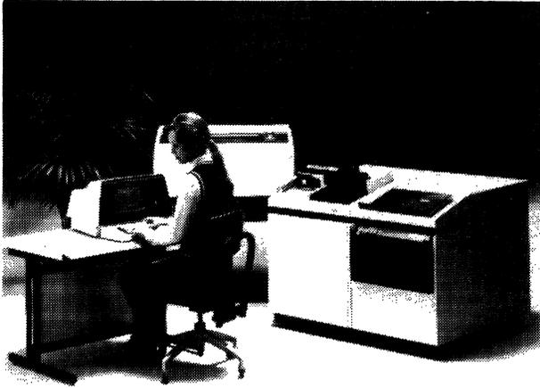
The Pertec XL40 is a disk-based system that can support both local and remote keystations.
