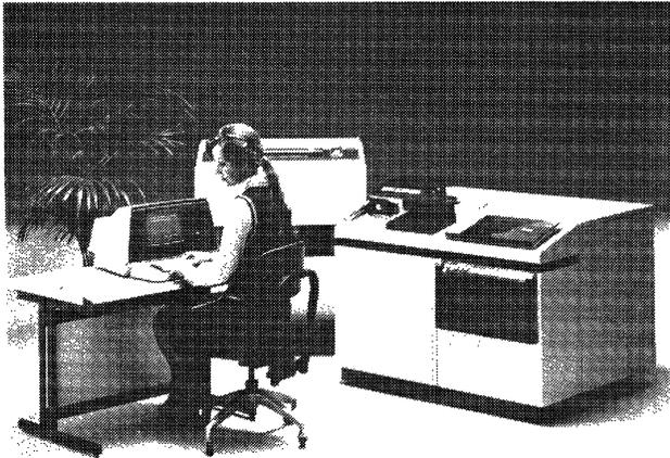
*The Pertec XL40 is a disk-based system that can support both local and remote keystations.*
