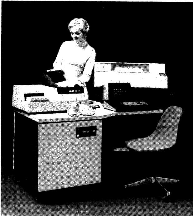
*The MDS 2300 shown above is equipped with the optional card reader, cartridge tape drive (directly beside the card reader), and line printer. This is a popular configuration for remote job entry.*
