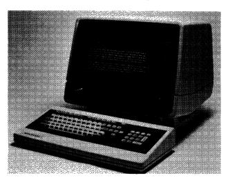
A new ergonomically designed keyboard/display was designed for use with Four Phase's Series IV/80 and IV/95 systems. The new unit features a redesigned keyboard, palm rests, tiltable screen with anti-glare filter, optional amber character read-out (green read-out is standard), and a new charcoal and white cabinet.
