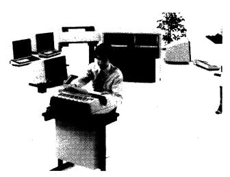
Four-Phase's new System 1V/60 features high processing speeds and total compatibility with existing Four-Phase software including the new Multifunction Executive Positioned as a mid-range processor, a 1V/60 with 192K bytes of main memory can support up to 24 1920-character video terminals, up to 22.5 megabytes of disk storage, and a variety of printers.
