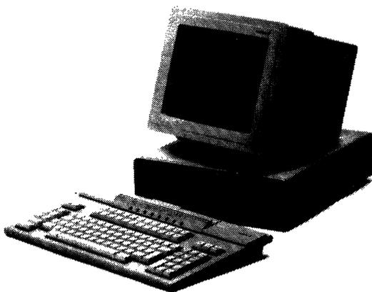
*The 3111 Workstation shown is one of 5 display unit models in the Alfaskop System 41. All models can be connected to a range of host computers, including IBM and Sperry machines.*
