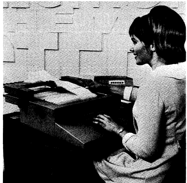
The Nixdorf 820/03 Terminal Computer is one of numerous models in the Series 800. Manufactured in West Germany, the Series 800 machines feature both core and “rod cell” storage, plus microprogrammed logic.
