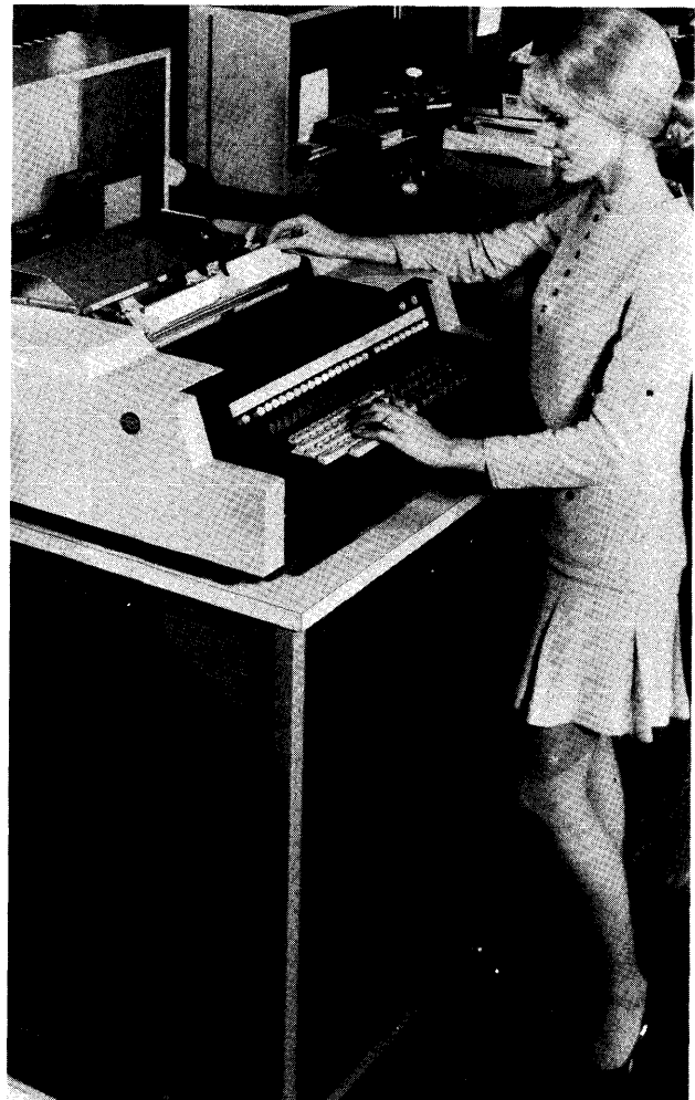
The Burroughs L 3000 Window Accounting Computer, like other models of Burroughs' popular L Series accounting computers (and their communications-oriented TC Series counterparts), features a magnetic disc memory that holds data, the user's programs, and "firmware" (microprogramming) that controls the system's arithmetic and logic operations. The L 3000 can accommodate passbooks for local operations as well as an interface to a central computer for on-line applications. With communications, the L 3000 is called a TC 700 Data Communications Terminal.
