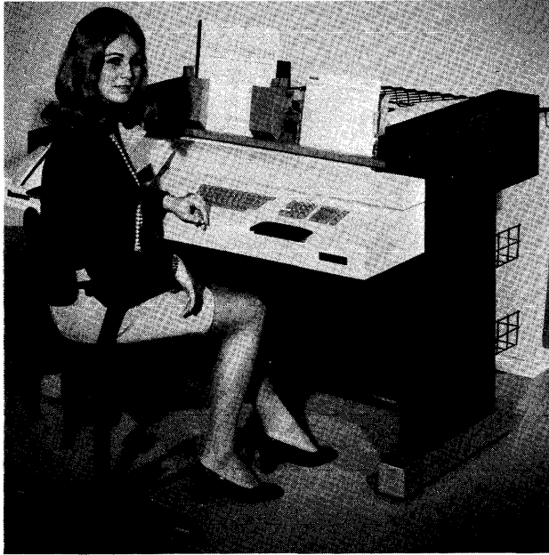
The Philips P-350 Series Office Computers feature 400 to 1200 15-digit words of core storage for both programs and data. The larger models can accommodate as many as 16 peripheral devices, up to 4 of which can operate simultaneously. Several thousand P-350 systems have already been sold in Europe.
