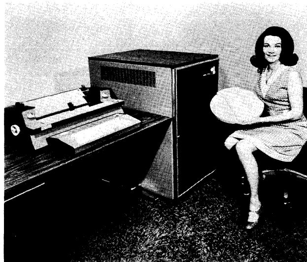
The Basic/Four computer systems are built around a Microdata 1600 minicomputer and feature a replaceable-cartridge disc memory that holds from 2.1 million to 12.6 million bytes. The BASIC programming language is supported, and up to 8 interactive terminals can be connected to the system.
