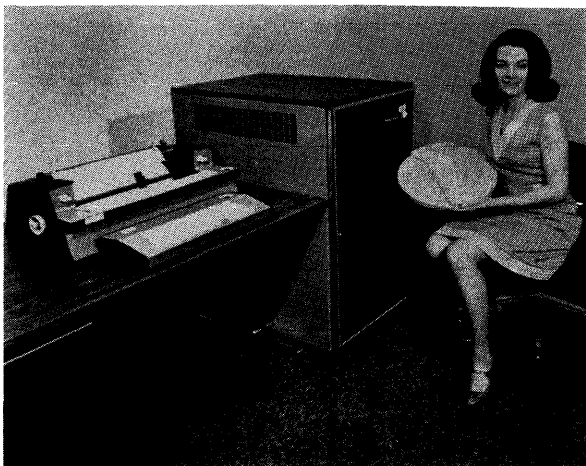
The Basic/Four computer systems are built around Basic/Four's own minicomputer and feature a replaceable-cartridge disc memory that holds from 2.1 million to 12.6 million bytes. The BASIC programming language is supported, and up to 8 interactive terminals can be connected to the system.
