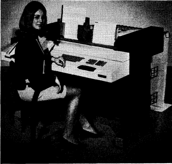
The Philips P-350 Series Office Computers feature 400 to 1200 15-digit words of core storage for both programs and data. The larger models can accommodate as many as 16 peripheral devices, up to 4 of which can operate simultaneously. Several thousand P-350 systems have already been sold in Europe.
