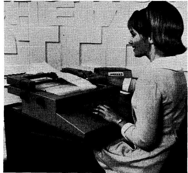
The Victor 820/03 Terminal Computer is one of numerous models in the Series 800, manufactured by Nixdorf in West Germany and sold and serviced by Victor Comptometer in the United States. The Series 800 machines feature both core and "rod cell" storage, plus microprogrammed logic.
