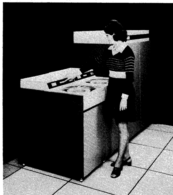
The large-capacity Model 8433 "double density" Disk Pack Drive, which stores up to 200 million bytes, is one of three new random-access storage devices announced for use with all the UNIVAC 1100 Series computer systems in March 1975. An 8433 Disc Drive Subsystem has a capacity of 1.6 billion bytes, or 3.2 billion bytes with the 16-Drive Expansion Feature. The 8433, the new 8405 Fixed-Head Disc Drive, and the 8430 (100-million-byte) Disc Pack Drive can be intermixed on a new microprogrammed control unit.
