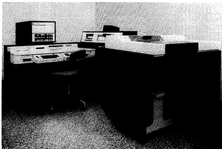
The Honeywell Model 58 combines a central processor, alphanumeric and numeric keyboards, card reader, and optional card punch in a single compact unit. The free-standing line printer is shown at the right.
