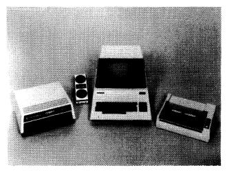
The Commodore CBM Business System depicted above consists of a fully-integrated CPU with built-in CRT, 32KB RAM memory, 18KB ROM, a typewriter-style keyboard, and a 10-key pad for rapid numeric entry. Peripherals include 51/4" dual diskette drive, 65 cps printer, and 300 bps modem.
