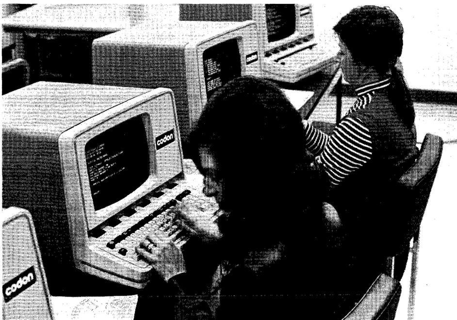
*The human side of CB-100 activity takes place primarily at the Video Data Terminals where clerks key in data and observe system messages on the screen. Not shown are the various printers, which also provide important system output, or the minicomputer processor and disk drives.*
