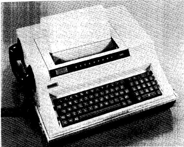
*The Execuport 300, produced by Computer Transceiver Systems, Inc., is a portable typewriter terminal that weighs 29 pounds, contains an acoustic coupler, and features a non-impact matrix printer rated at 10, 15, or 30 characters per second. CTSI boasts that over 3000 of these units have been delivered. Respondents to Datapro's user survey were well pleased with the Execuport 300's performance.*
