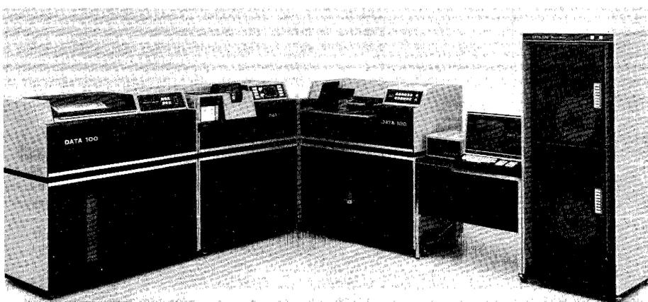
*DATA 100's Model 78 Terminal is programmable and can include up to 12 I/O devices. This configuration includes (left to right) a printer, card reader, punch, operator console (CRT display), and computer-compatible magnetic tape unit containing two drives.*
