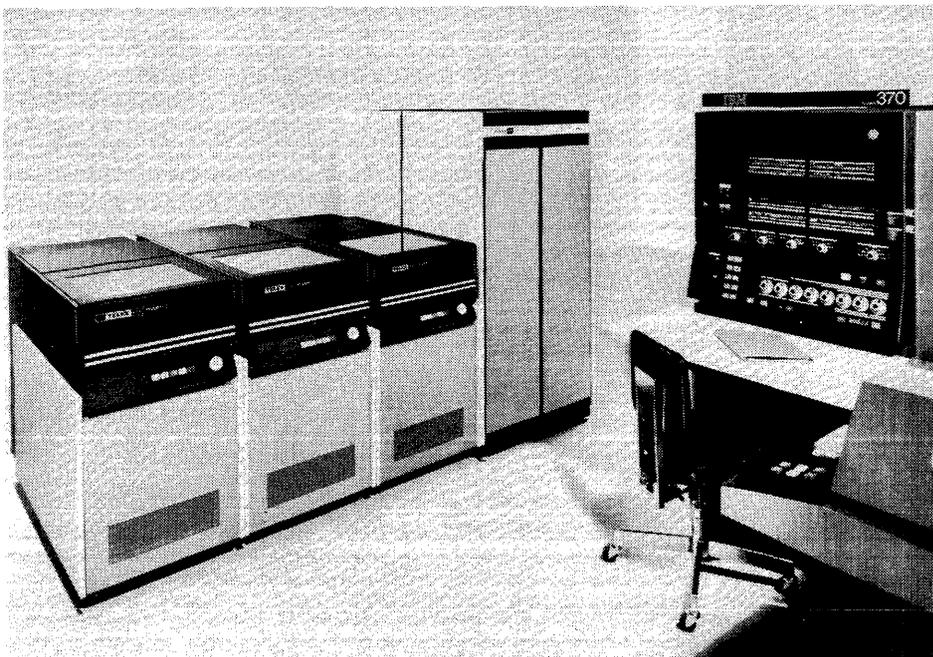
*In contrast to the IBM 3330 packaging, each of the Telex 6316 disk drives is housed in a separate cabinet. The Telex controller is in the center.*
