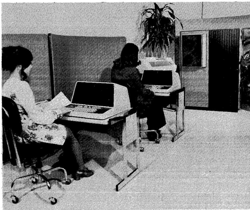
*A Key-Edit 50 system can include from 4 to 16 of the CRT keystations shown in the foreground. At rear are the central unit, which houses the processor, fixed-head disk unit, and optional 165-cps matrix printer.*
