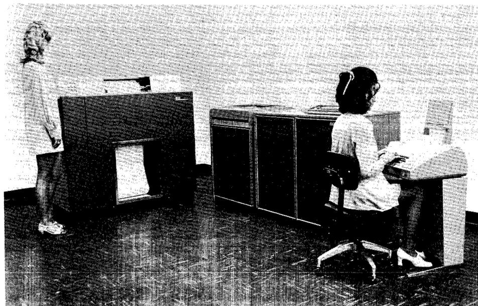
*The DataPrint System couples the widely respected IBM 1403-N1 Printer (left) with a minicomputer-based control unit, a supervisory teleprinter, and from one to eight magnetic tape drives.*
