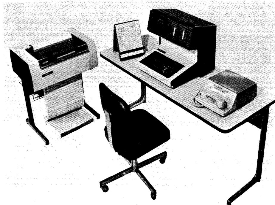
*The basic Sycor 340 Terminal contains a microprocessor, CRT display screen, keyboard, and one or two cassette tape recorders. This system, configured to handle branch-office data entry and communications functions, also includes a 30-cps printer (at left) and a data communications interface.*
