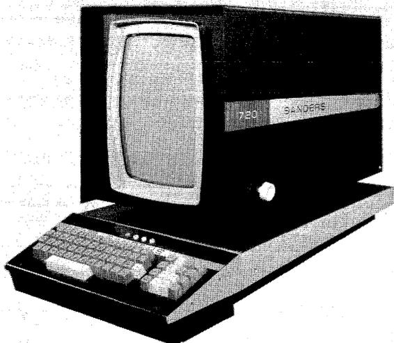
The Sanders 720 is a multiple-display, multiple-printer video display system designed for local or remote operation with a computer. Sanders provides an interface and buffering arrangement for use with an IBM System/360. A wide range of display configurations is available.
