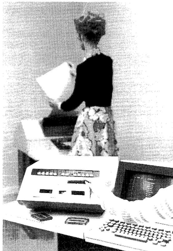
UNIVAC's Model 610 Tape Cassette System adds useful remote batch or off-line data handling capabilities to the Uniscope 100 or 200.
