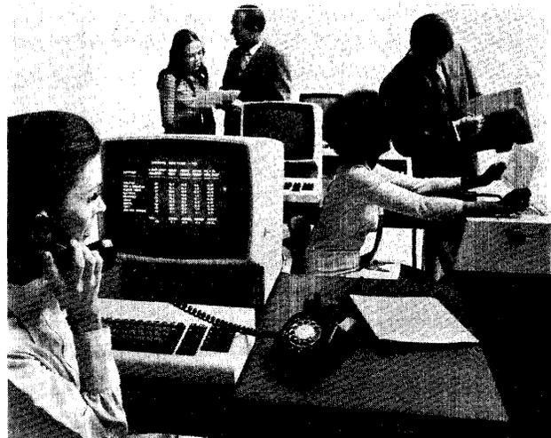
*Surprise! IBM is in first place – this time in the CRT display terminal market with the 3270 Information Display System. The display is useful, but it's the keyboard that enables data to be transmitted directly to a computer via communications links. Hence, it's the keyboard that makes the CRT terminal an attractive data entry device.*
