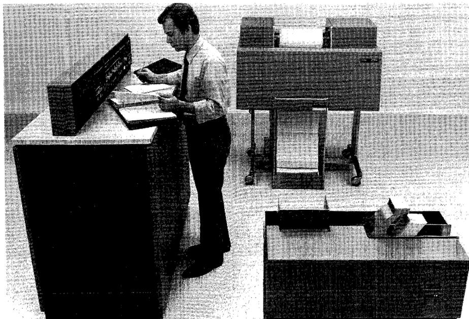
*This view of the 2922 Programmable Terminal clearly indicates its 360/20 origins. The controller is at left, with 500-cpm card reader in the foreground and 500-lpm chain printer at rear.*
