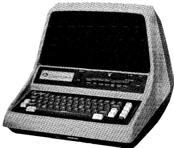
The Executerm I is a low-priced interactive terminal that offers Teletype compatibility, selectable transmission speeds up to 1200 bits/second, and editing capabilities. Options include a parallel interface and an impact printer.
