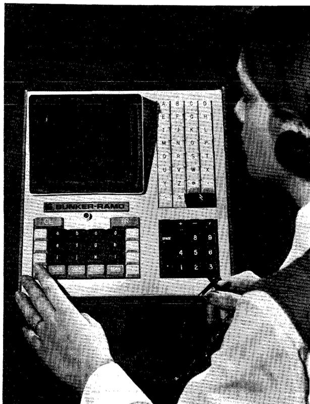
The Bunker Ramo Model 2212 Display Station, a small desktop unit, contains a 6-inch CRT and an alphanumeric keyboard arranged for non-typists. The Model 2210 Display Station is similar in appearance, but contains a 3-inch CRT.
