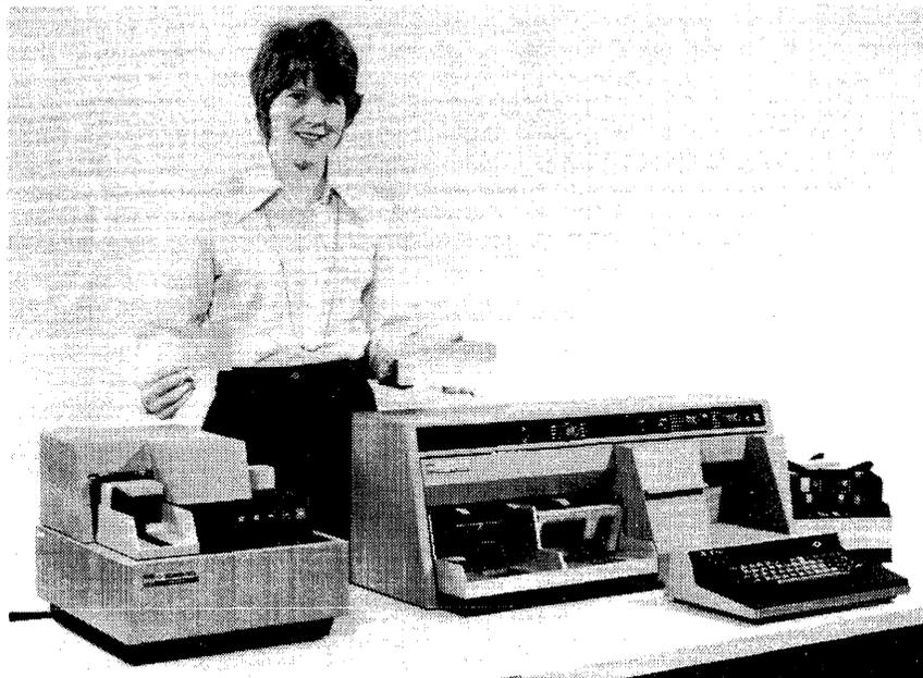
*This Decision Data 8010 Interpreting Data Recorder is shown with the optional 96-to-80-Column Card Converter (at left). The 8010's dual input hoppers can be seen at the far right, while the dual output stackers are clearly visible to the left of the keyboard.*
