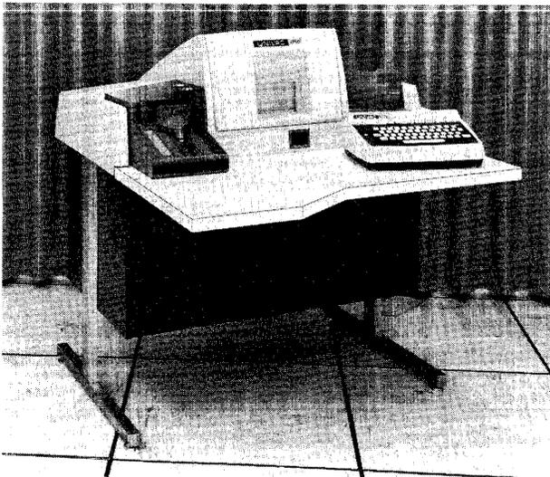
*The widely used UNIVAC 1710 VIP keypunch is one of several units on the market today that boast of electronic operation and data buffering. In addition to its role as a keypunch, the 1710 also acts as a verifier and an interpreter.*
