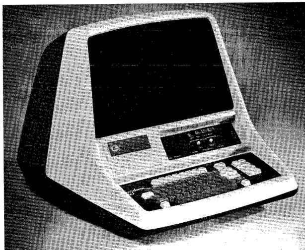
*The Executerm 260 replaces the IBM 2260 Display Station and has a display capacity of either 960 or 1920 characters. The Executerm 60, 65, and 265 terminals are quite similar in appearance.*
