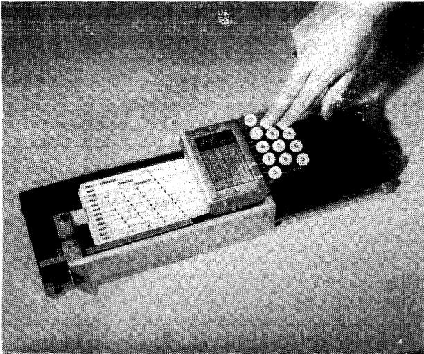
*It looks simple, and it is. The Wright Line Punch can produce any card code by simply depressing as many keys as required. It may not be fast, but it doesn't require anything but a tab card and an operator to produce computer input.*
