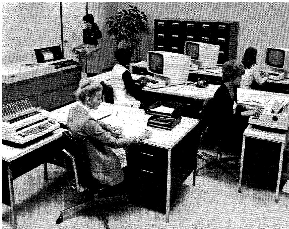
*This typical 3790 system installation demonstrates the operating flexibility that can be derived by mixing 3277 Display Stations and 3793 Keyboard-Printers to serve various business applications. The 3791 Controller with line printer is shown at the left.*
