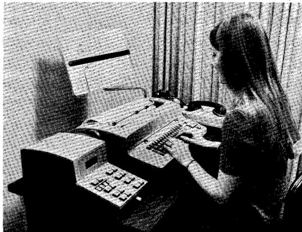
*The Trendata Model 1500, an IBM Selectric-based terminal that features an added tape cassette unit and acoustic telephone coupler, is a replacement for IBM's own 2740-1 Communications Terminal.*
