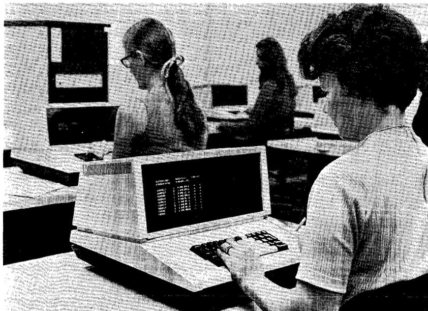
*The Scan-Data 2250/2 Key Entry System can support as many as 32 of the Scan-Plex II CRT display keystations shown here. When an optical scanner is added, the resulting configuration is known as a 2250/3 Mixed Media System.*
