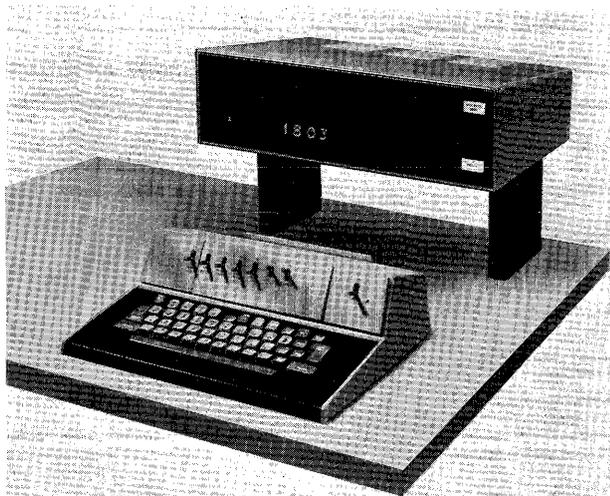
The CMC 11 display panel is informing the operator that the character just entered was an "x" and that the station is in the Data Entry mode and is ready to accept the next entry, which will be the third character in the eighteenth field of the record.
