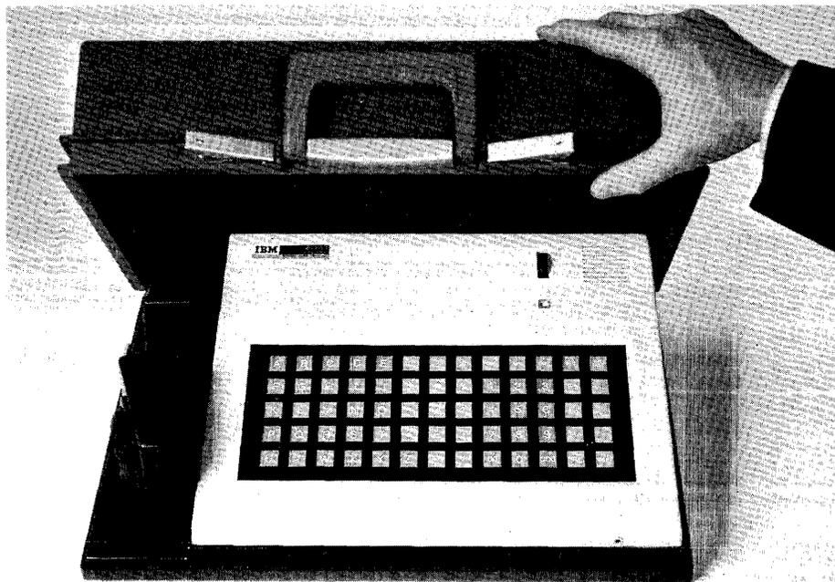
*The 2721 Portable Audio Terminal has a highly unorthodox "flat" keyboard, as well as an unconventional key arrangement designed for convenient use by nontypists.*
