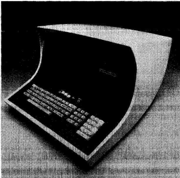
This modern display terminal produced by Applied Digital Systems (ADDS) is available as a Teletype replacement (Model Data 980) or an IBM 3275 replacement (Model 980A). Features include a 1920-character screen, full edit and data entry capabilities, and numeric keypad.
