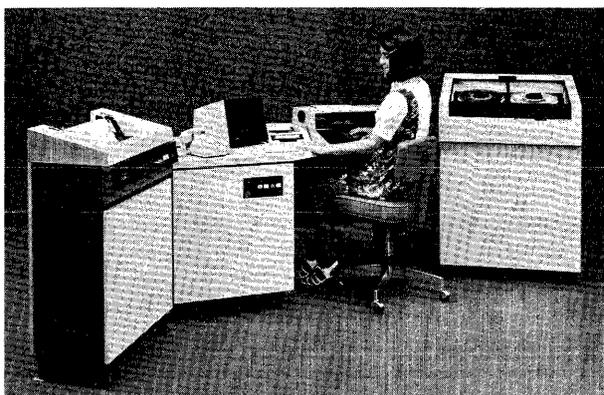
The basic 2307 Control Unit at center, with its CRT display and keyboard/printer, is flanked by the optional 100-cps matrix printer at left and a 9-track magnetic tape drive at right. Also housed in the compact control unit are a 4K-byte minicomputer and disk drive.
