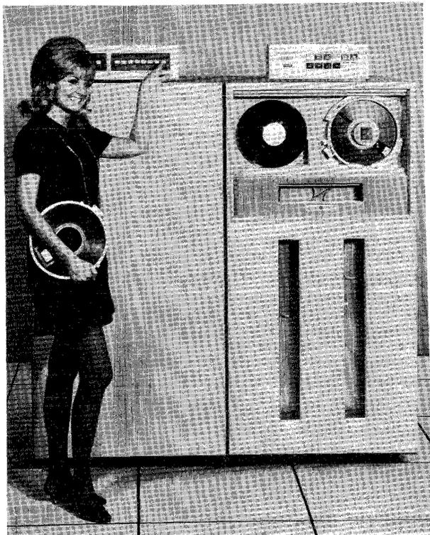
CalComp's 1040 System is a high-performance plug-to-plug replacement for the IBM 3803/3420 Magnetic Tape Subsystem. Although new to the plug-compatible tape community, CalComp is a major supplier of IBM-compatible disk drives.
