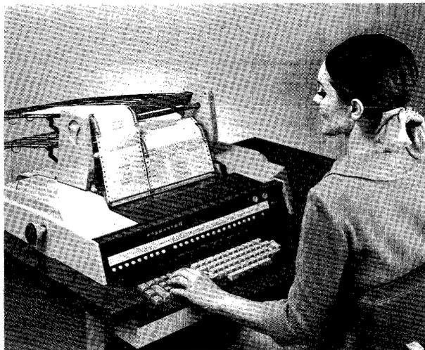
The TC 500 carriage is capable of feeding two side-by-side continuous forms. The keyboard includes a typewriter-style key-group, a numeric keygroup, and a long row of control keys and indicator lights.
