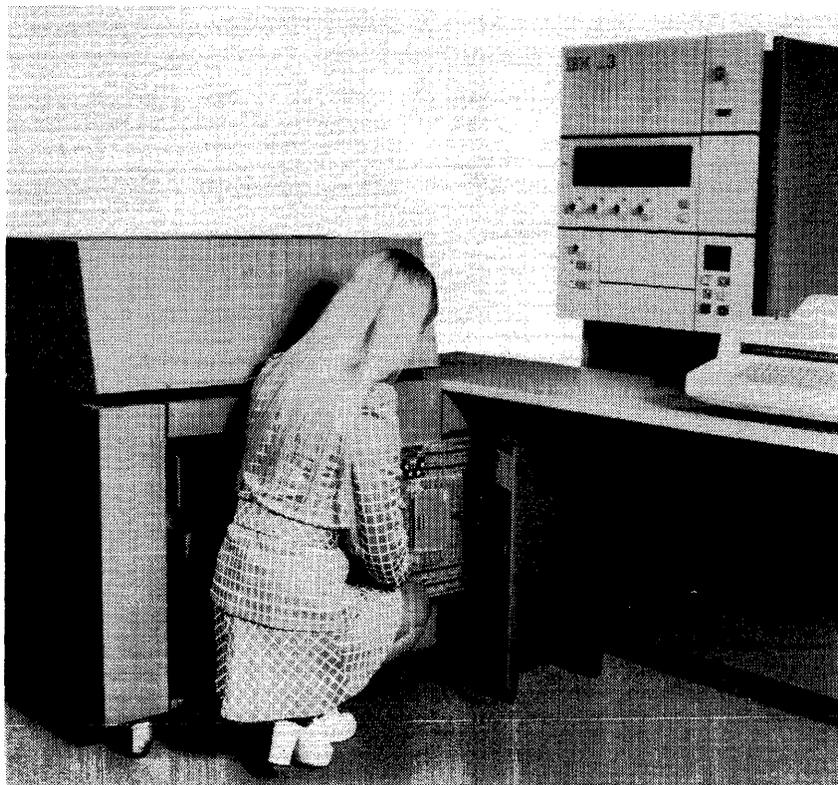
*Up to 56K bytes of BST/3 core memory fits neatly beneath the System/3 operator console as shown here.*
