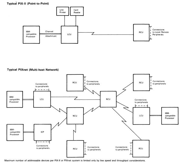
Maximum number of addressable devices per PIX-II or PIXnet system is limited only by line speed and throughput considerations. Maximum number of other control units directly attachable to NCU is 13.
