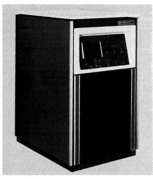
The PIX Remote Control Unit (RCU) is located remotely to the host computer and communicates with the host via a PIX Local Control Unit (LCU). A variety of peripheral devices/ controllers can be physically connected to an RCU. The maximum number of terminal devices that can be connected to an RCU is 96.
