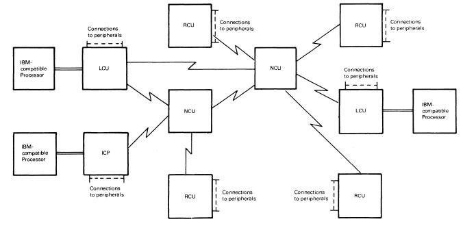
Maximum number of addressable devices per PIXNET system is limited only by line speed and throughput considerations. Maximum number of other control units directly attachable to NCU is 13. Maximum number of devices (peripherals or other control units) directly attachable to LCU depends on types of devices and line speeds.
