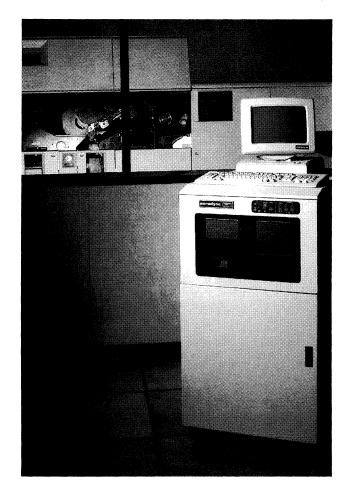
Paradyne's PIXNET/XL allows remote peripherals to function as if they were in the same room with the host. This system supports up to 384 terminals.
