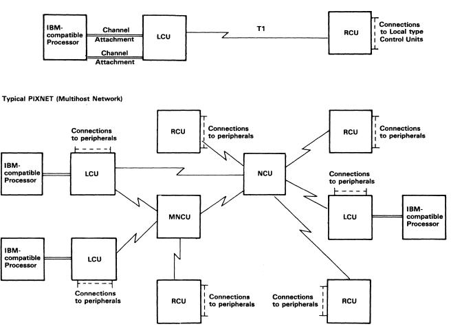
Maximum number of addressable devices per PIXNET system is limited only by line speed and throughput considerations. Maximum number of other control units directly attachable to NCU is 13.
