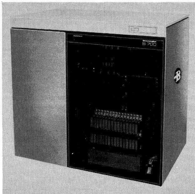
The B 774 front end accommodates up to 32 communications lines for Burroughs computer systems. It can also be used remotely for line concentration and control functions. Its application is limited to the Burroughs generated communications control microcode.
