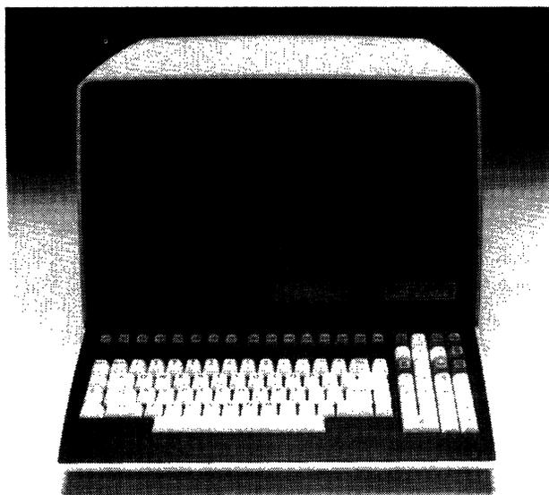
Introduced in late 1979, the Zentec Zephyr can generate and display 128 ASCII characters, and can transmit data in character, line, or block format at speeds from 110 up to 19,200 bps.
