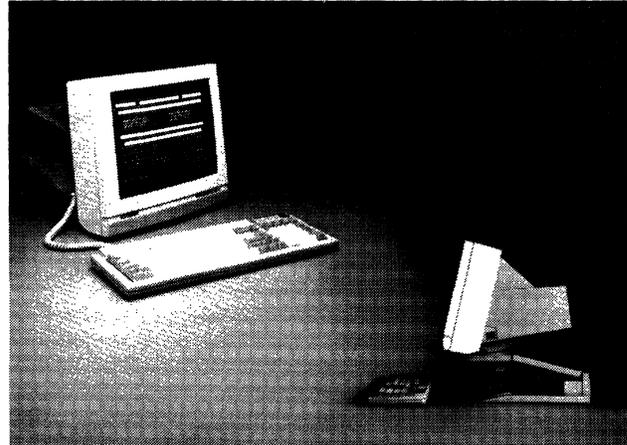
*The new WY-30 contains smart terminal features and carries a purchase price of \$399. The terminal includes a 14-inch display with a touch-tilt mechanism; a height-adjustable arm, shown here at the lower right, is optional.*
