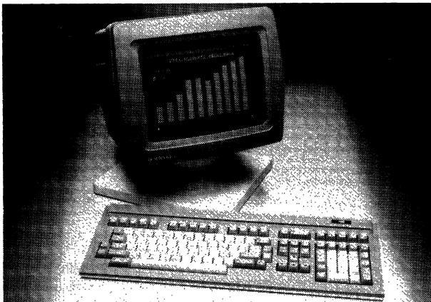
*TeleVideo's new Model 922 is a DEC VT220 emulator that sells for \$995 (list price). The 922 features a 12-inch display screen with 80-/132-column display capability. The keyboard is detachable, has a low-profile design, and boasts some key layout improvements over the DEC VT220 keyboard.*
