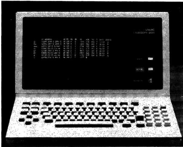
UNIVAC offers a wide choice of keyboard arrangements for the Uniscope terminals. The Uniscope 200 shown here has both a typewriter-style alphanumeric keygroup and a separate numeric keygroup (at right).
