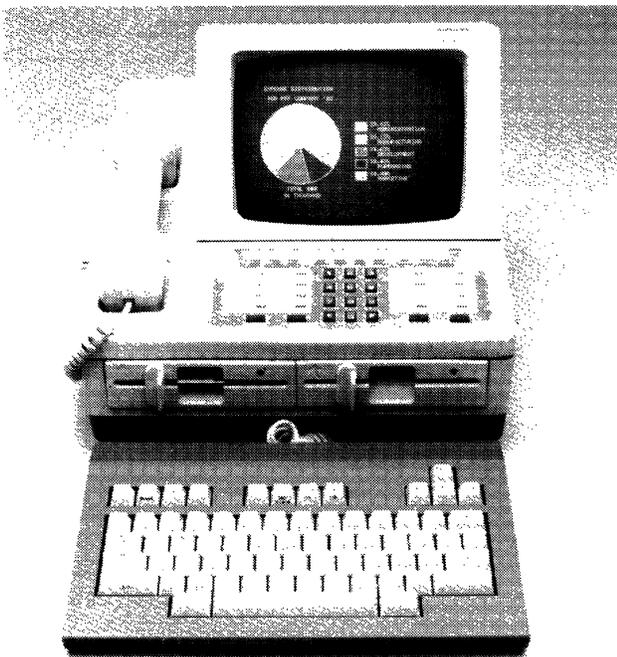
*The Rolm Cedar is an IBM PC-compatible integrated voice/data workstation. Features include a 9-inch display, retractable alphanumeric keyboard, integrated handset with speakerphone, two diskette drives, and 512K bytes of memory.*
