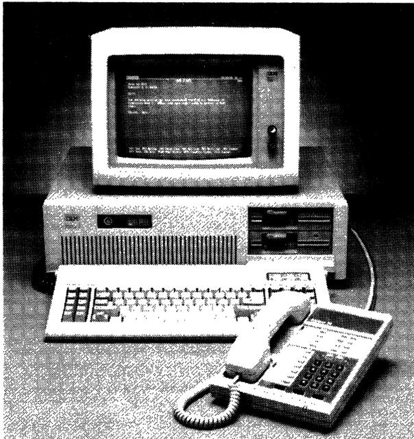
*Juniper II is an IVDT enhancement product designed for use with the IBM Personal Computer family. The Juniper II consists of a specially designed ROLMphone 240, cable connection to the PC, Rolm Personal Communication Software, and a plug-in option card that occupies a single slot in the PC. The Juniper II is shown here connected to an IBM PC AT.*
