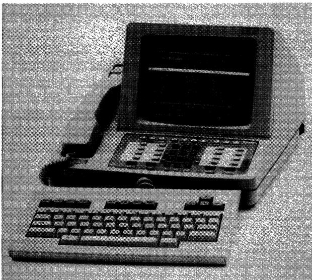
*The Rolm Cypress terminal is an integrated voice data terminal. Features include a 9-inch, retractable alphanumeric keyboard, an integrated handset with speakerphone, and personal communications software that improves productivity.*
