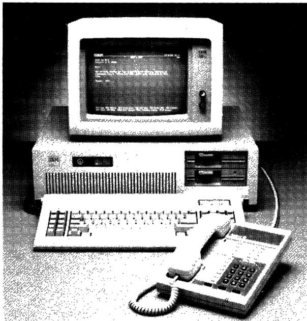
*Juniper II is an IVDT enhancement product designed for use with the IBM Personal Computer family. The Juniper II consists of a specially designed ROLMphone 240, a cable connection to the PC, Rolm Personal Communication Software, and a plug-in option card that occupies a single slot in the PC. The Juniper II is shown here connected to an IBM PC AT.*
