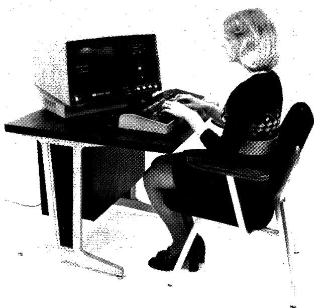
*Control Data's new, microprocessor-based Model 92451 Conversational Display provides Teletype Model 33/35 compatibility and features a 960- or 1920-character screen and a host of options. Auxiliary devices include a single- or dual-drive diskette or cassette tape unit and a 180-cps impact or 30-cps non-impact printer. The OEM base price is \$2,000; quantity discounts are available.*
