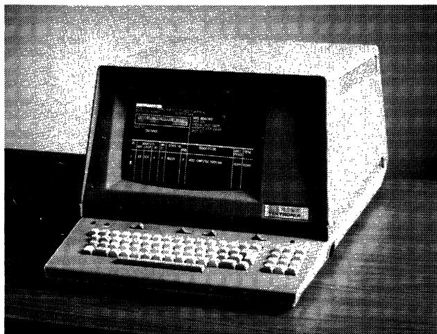
Here's an example of the use of partial reverse video (dark characters on light background) and formatted operation. The Tektronix 4023 is a general-purpose alphanumeric terminal with a 12-inch CRT, capable of displaying up to 1920 characters. Options include the Ruling Character Set (shown above as the solid horizontal and vertical lines), a hard-copy unit (Model 4023), and a cartridge tape drive (Model 4923). Tektronix is a leading vendor of graphic display terminals.
