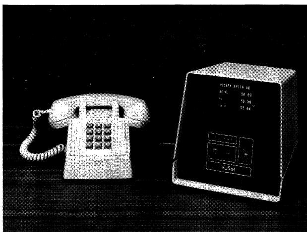
*Plantronics's VuSet, available from the Bell System for \$35 per month, provides a 3-inch CRT that displays any of 64 characters in up to 64 display positions. It's intended for applications that involve short messages such as account status, sales statistics, customer balances, etc. The VuSet attaches to any Touch-Tone telephone, which is used to call the computer and to enter data; a VuSet modem is required at the computer end.*
