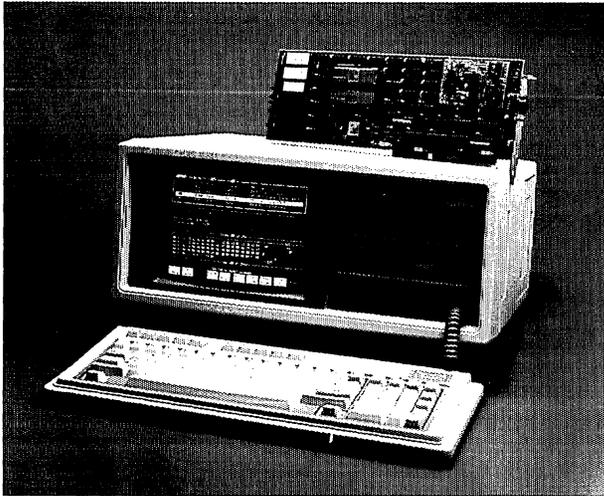
*The Sniffer, from Network General, is the most popular LAN diagnostic device on the market today. The Sniffer provides diagnostic capabilities for Ethernet, token-ring, ARCnet, IBM PC Network, Starlan, and LocalTalk LANs.*
