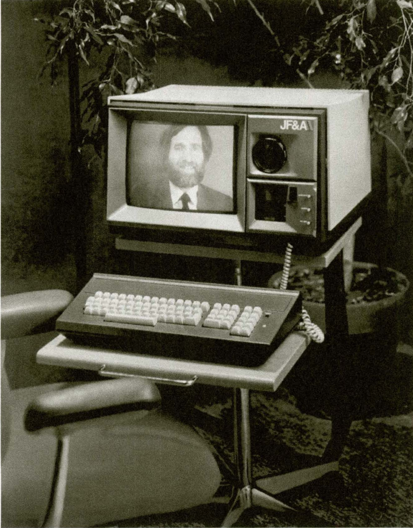
JF&A1, one of five prototype videoconferencing systems developed by John Frassanito & Associates, David Monroe U.S. Patent number 4,710,917, 4,847,829.
