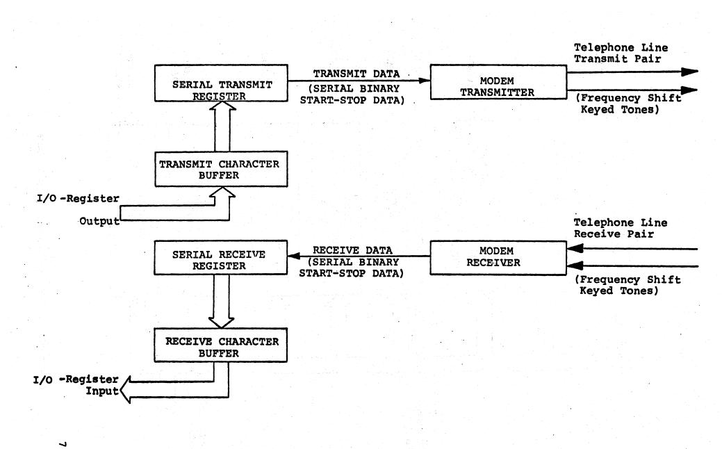
FIGURE 3-1 9402 BASIC FUNCTIONAL DIAGRAM
