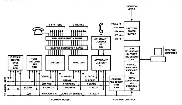
Figure 1 • Harris 400/1200 System Block Diagram.
