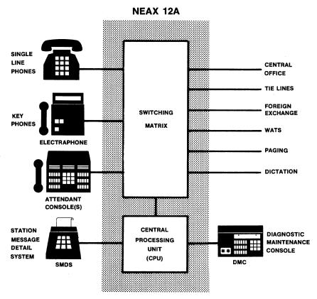
Figure 1 • NEAX 12A block diagram.
