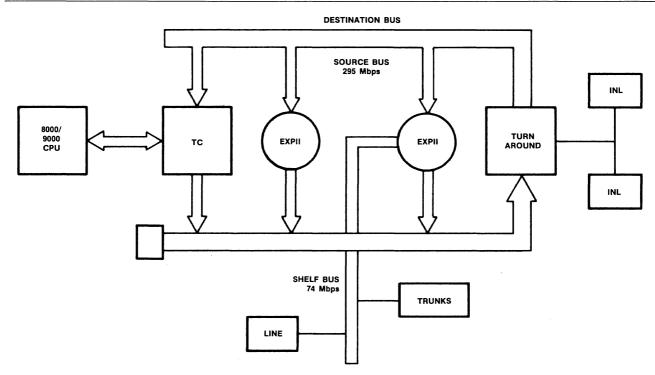
Figure 3 • Rolmbus 295 configuration. The intershelf bus (Rolmbus 295) consists of 2 unidirectional buses (source and destination buses). Expander II cards interface the source and destination buses to the shelf bus, which runs at 74 Mbps and is Rolmbus 74 compatible. The TDM Controller (TC) card drives the Rolmbus 295 at 18.432 Mhz, while the Turn Around (TA) card serves to synchronize the Rolmbus 295 either intranode or internode across the Internode Link.
