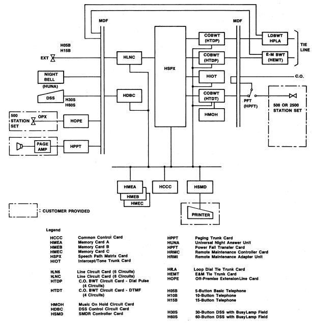
Figure 4 • Focus Hybrid Block Diagram
