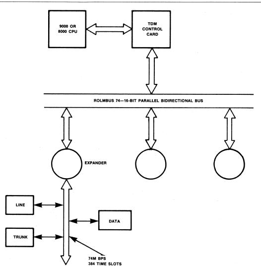
Figure 2 • Rolmbus 74 configuration. Lines, trunks, and data terminals are connected to expander via Rolmlink; 256K-bps slot is available for voice, data, and control signals. The connection to Rolmbus 74 is via expander; all system control functions are handled by 8000 or 9000 CPU connected to Rolmbus via TDM control card.
