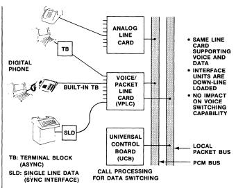
Figure 1 • Omni dual-bus architecture.
