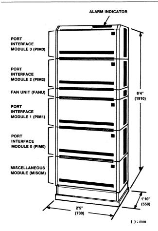
Figure 2 • NEAX 2400 interface module group (IMG).
