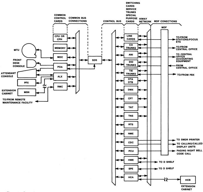
Figure 3 • Focus PBX Functional Block Diagram
