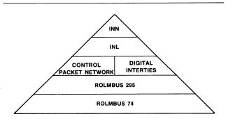
Figure 1 • CBX II Systems Architecture Hierarchy. CBX II architecture begins at the Rolmbus 74 level, for most current applications, and grows through the higher performance Rolmbus 295. Multinode applications tie together with the Control Packet Network and Digital Interties. Larger installations requiring substantial data capabilities build on Inter-Node Links and Inter-Node Network.
