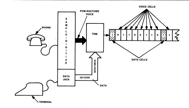
Figure 8 • digital data in a PCM-based digital PBX.
