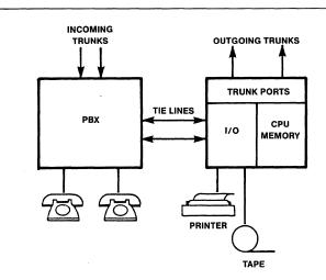
Figure 2 • Least Cost Routing System Configuration
