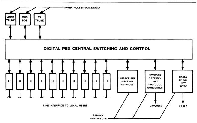
Figure 12 • service processors/gateways in a digital PBX.
