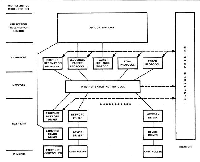
Figure 4 • Architecture of the ITP protocol packages.
