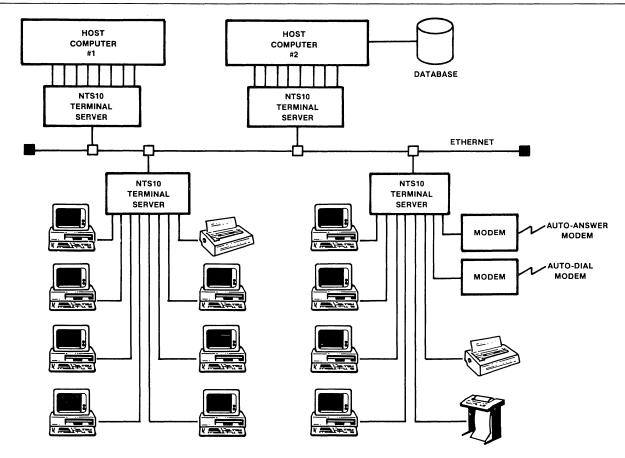
Figure 3 • With poly-TRM and poly-XFR, the NTS10 Terminal Server provides PC-to-Host, PC-to-PC, and PC-to-Device communication.
