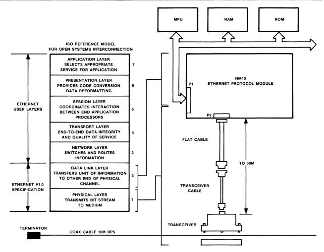
Figure 2 • Ethernet architecture and implementation.
