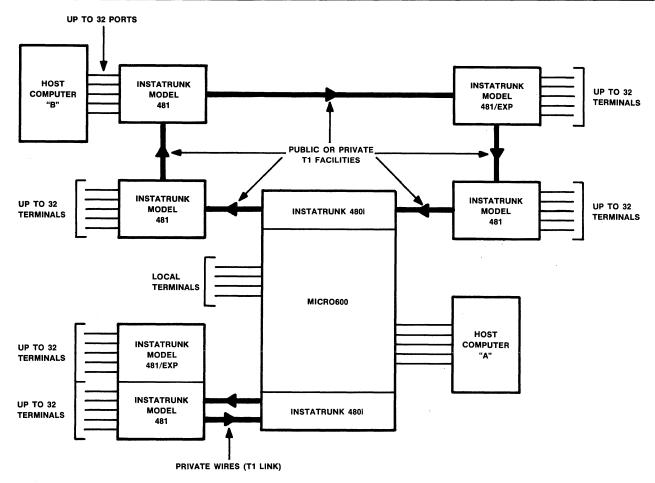
Figure 5 • Instatrunk remote bay/ring configuration.
