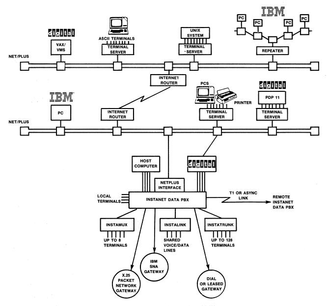
Figure 1 • Instanet/Plus integrates Micom's data PBX with Interlan's cable-based LAN.
