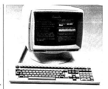
The new ADM 12plus terminal features a 24-line  $\times$  80-/132-column display format; up to 4 pages of display memory, and 16 programmable function keys (shiftable to 32 functions).
