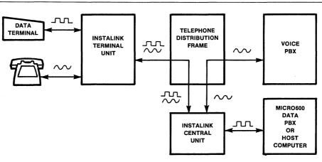
Figure 6 • Instalink 460 voice/data multiplexer.
