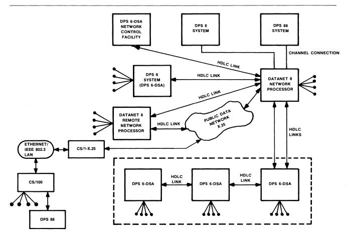
NOTE: ● = Terminal interfaces for async/sync devices including PCs running PC 7800 software to emulate VIP 7800 terminal. Figure 1 • typical DSA network configuration.
