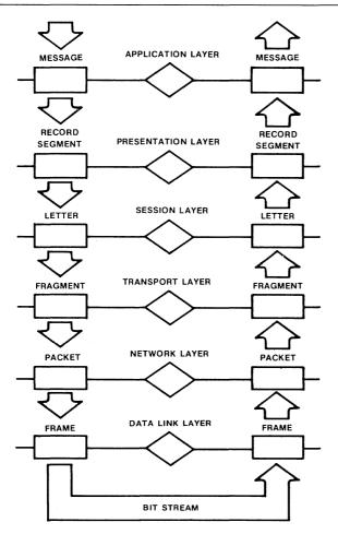
Figure 4 • units of exchange between DSA layers.
