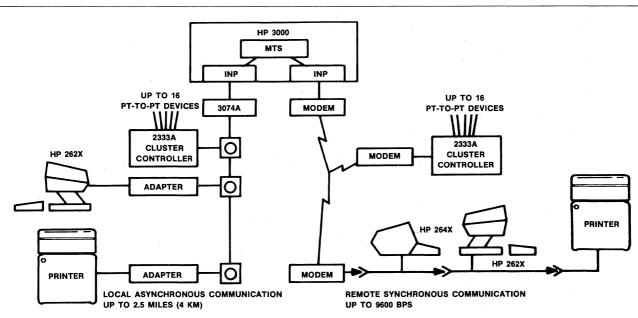
Figure 11 • Multipoint Terminal Software (MTS) support on HP 3000.
