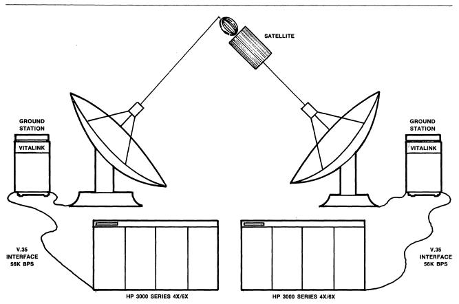
Figure 8 • satellite network link connecting HP 3000s.
