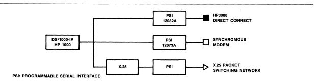
Figure 3 • DS HP 1000 to HP 3000 communication support.
