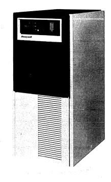
Datanet 8 Network Processor is the nucleus of Honeywell's Distributed Systems Architecture (DSA). It operates as a front-end network processor, network processor, and terminal concentrator.
