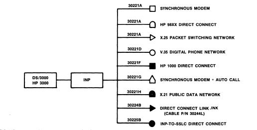
Figure 4 • DS HP 3000 to HP 3000 communication support.
