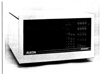
The CASE DCX840 addresses medium-to-large scale network requirements and can be configured with multiple composite network links for communicating with other DCX models in a multinode network.
