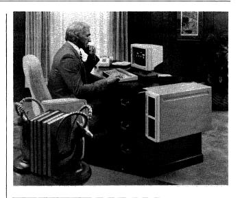
Mass Storage ● 360K-byte 5.25-inch diskette standard; either second 360K-byte 5.25-inch diskette or 10M-byte 5.25-inch hard disk can be added.
