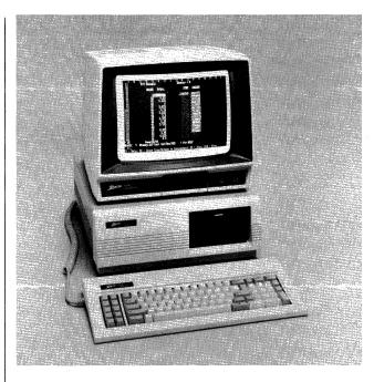
**Ports** • all models include 2 RS-232C asynchronous serial ports and a Centronics-compatible synchronous port.
