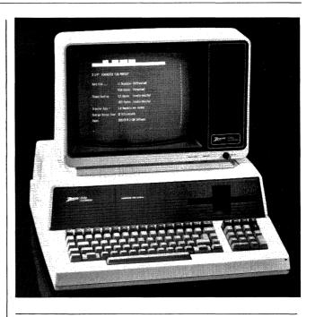
sor operating at 5 MHz and an 8-bit Intel 8085 microprocessor operating at 5 MHz.
