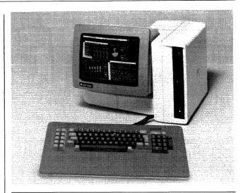
**Terminals/Workstations** • single-terminal systems with detached keyboard and integral disk drives; green tilt-adjustable monitor on desktop models; yellow integral monitor and composite video output on portable • local area network (LAN) facilities available from third-party vendors.
