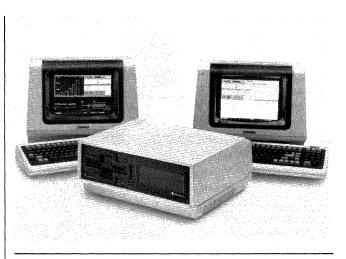
TS 804 comes with 320K bytes of RAM and 64K bytes of cache; TS 816/40 comes with 128K bytes of RAM.
