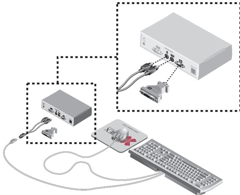
7. Connect the Category 5 cable to the modular jack on the rear of the Receiver.
