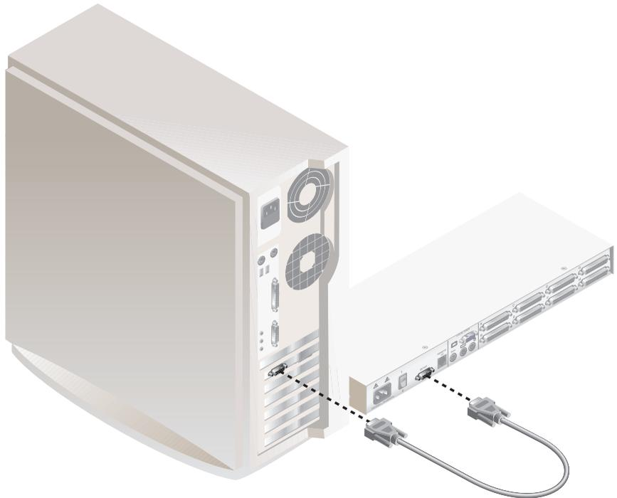
You will then need some form of terminal software on your attached computer so that it can communicate with the AutoView 400. There are several that are commercially available. Select one that you are comfortable with and be sure that it can communicate at 38,400 baud.
