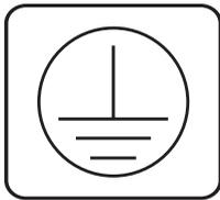
**PROTECTIVE GROUNDING TERMINAL:** A terminal which must be connected to earth ground prior to making any other connections to the equipment.
