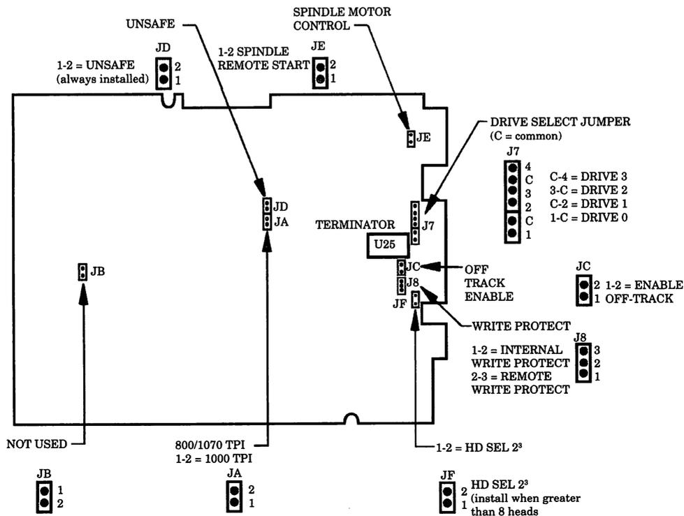
**Figure 17 – Maxtor XT 1000/2000 Series Drive Select Jumper Options**
