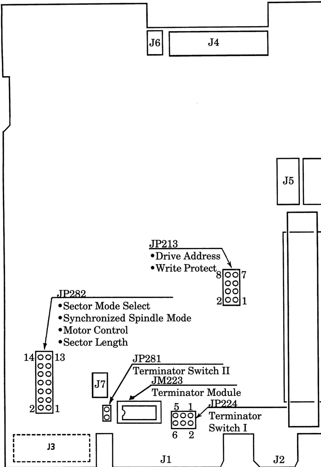
Figure 14 - SZ931 PCB Layout (Rev. 1 or later)
