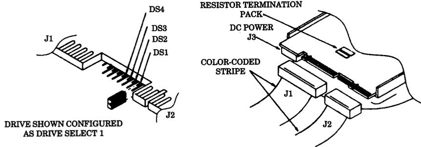
**Figure 27 – Half-Height Interface Connectors**
