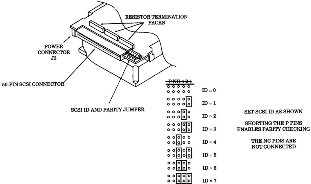
**Figure 30 – 3.5" SCSI Interface Connectors**
