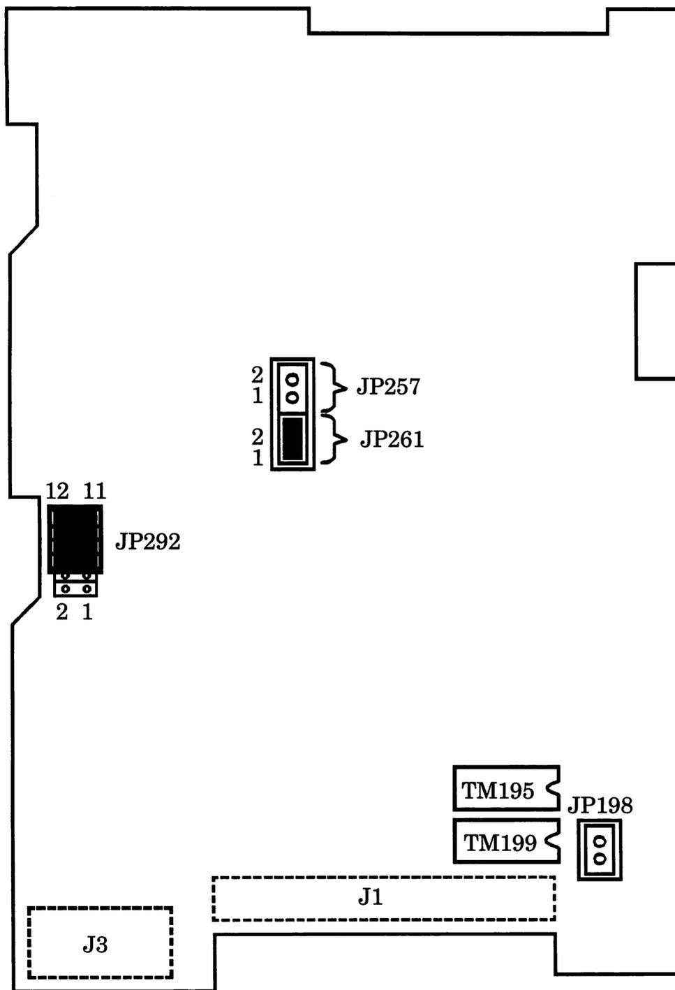
**Note:** The terminator of the DK514C must be removed except on the last drive of the Daisy Chain.
