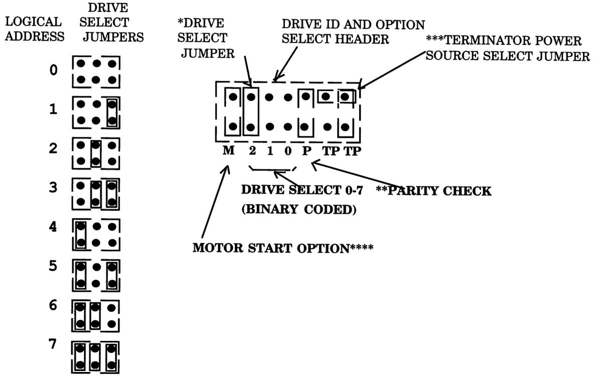
\* Drive ID is binary coded jumper position (most significant bit on left). i.e., jumper in position 2 would be Drive ID 4, no jumpers mean ID 0.
