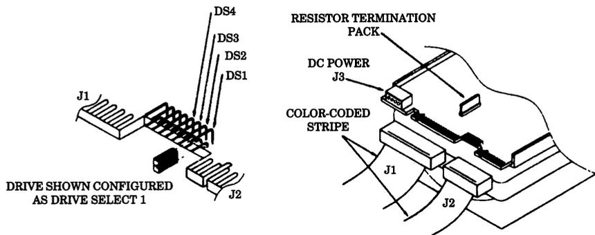
**Figure 28 – Full-Height Interface Connectors**
