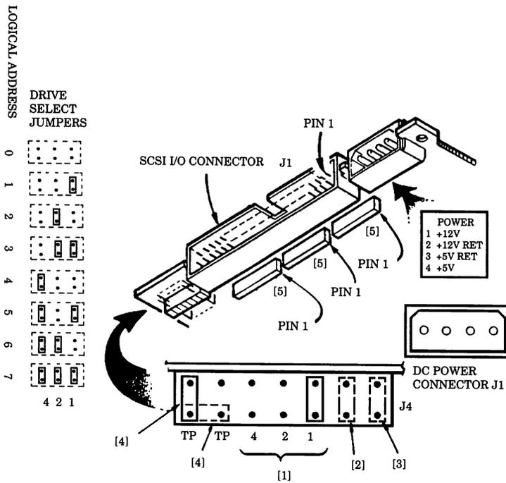
Figure 6 – CDC Wren V Series Jumper Location
