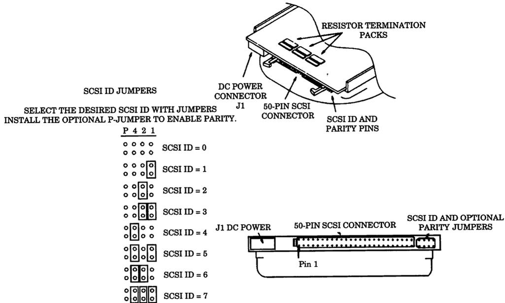
**Figure 31 – 5.25" SCSI Interface Connectors**
