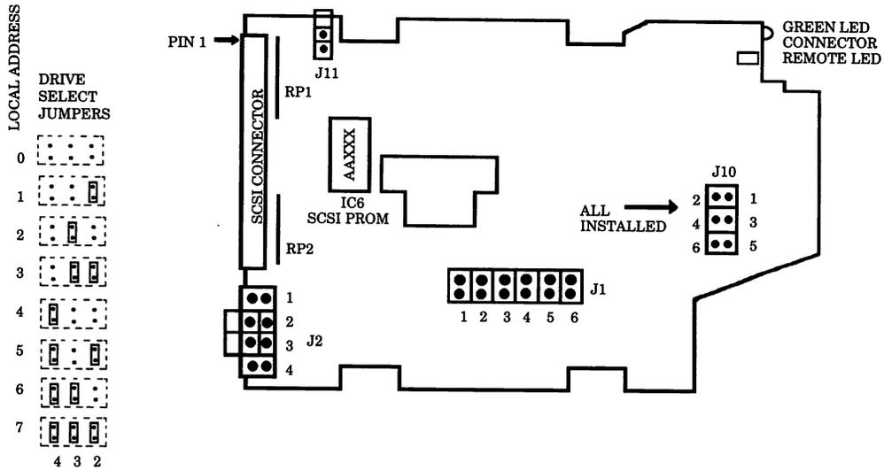
**Figure 15 - Maxtor LXT-100 Jumper Locations**
