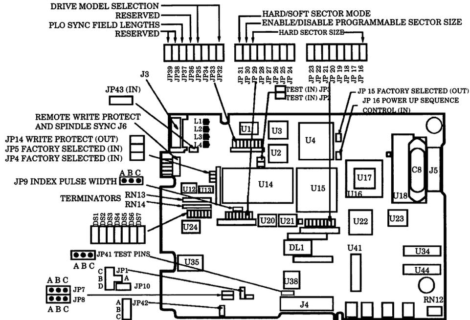
Figure 20 – Drive Jumper Options (PCB P/N 1015468)
