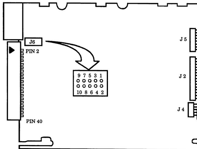
**Figure 16 - Maxtor LXT-200A PCB Layout**
