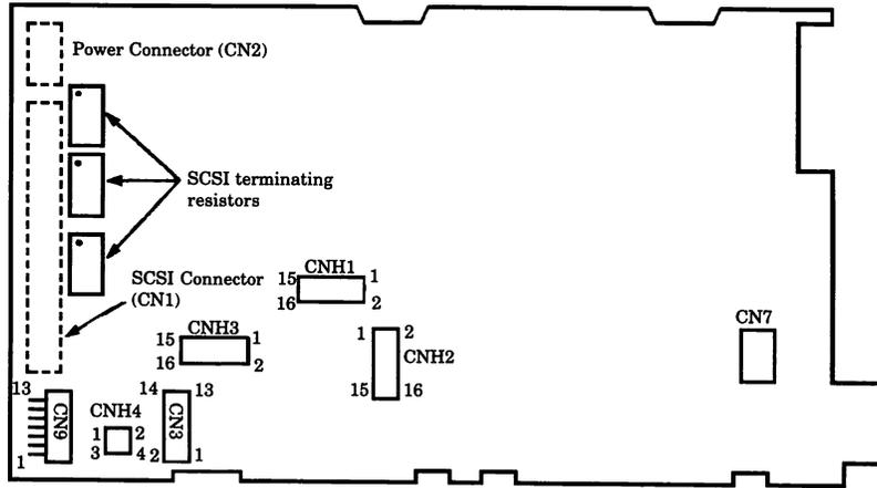
**Figure 8 – Fujitsu 226X Series Jumper Locations**
