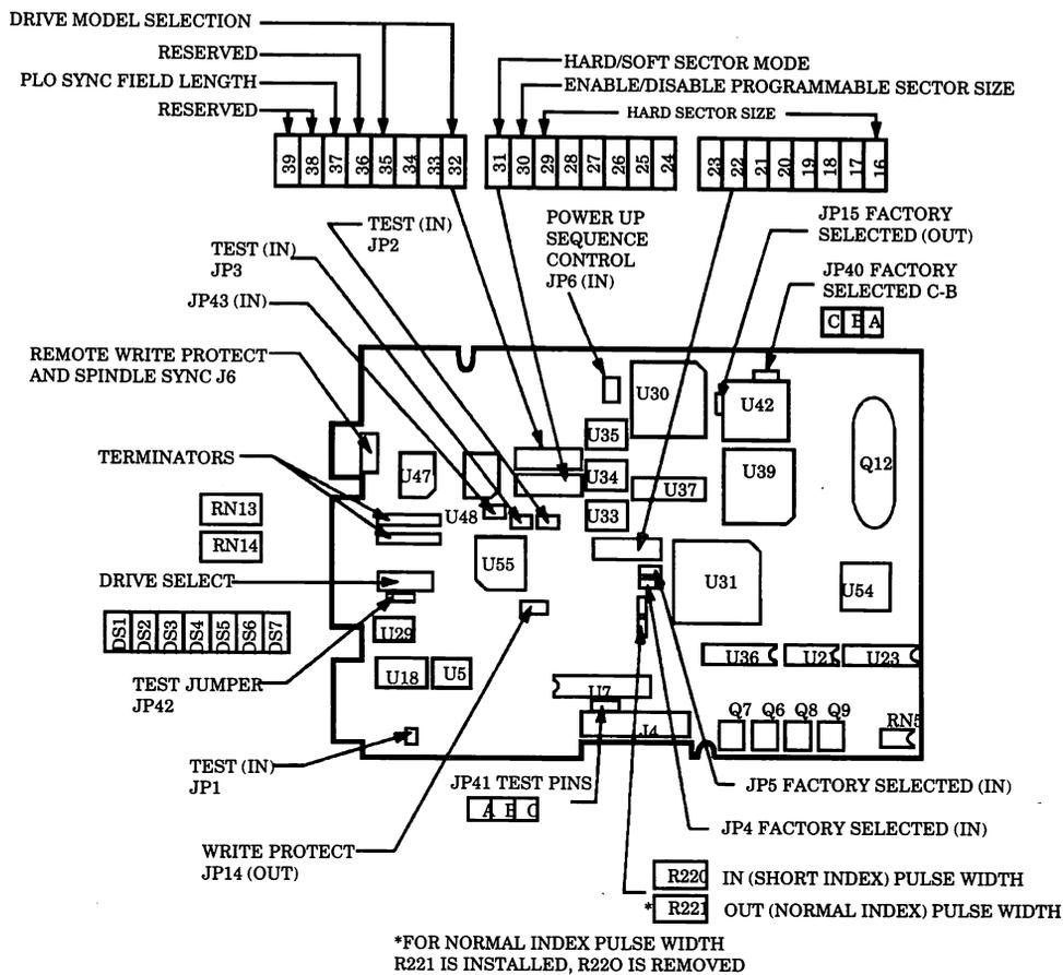
Figure 19 – Drive Jumper Options (PCB P/N 1014150)
