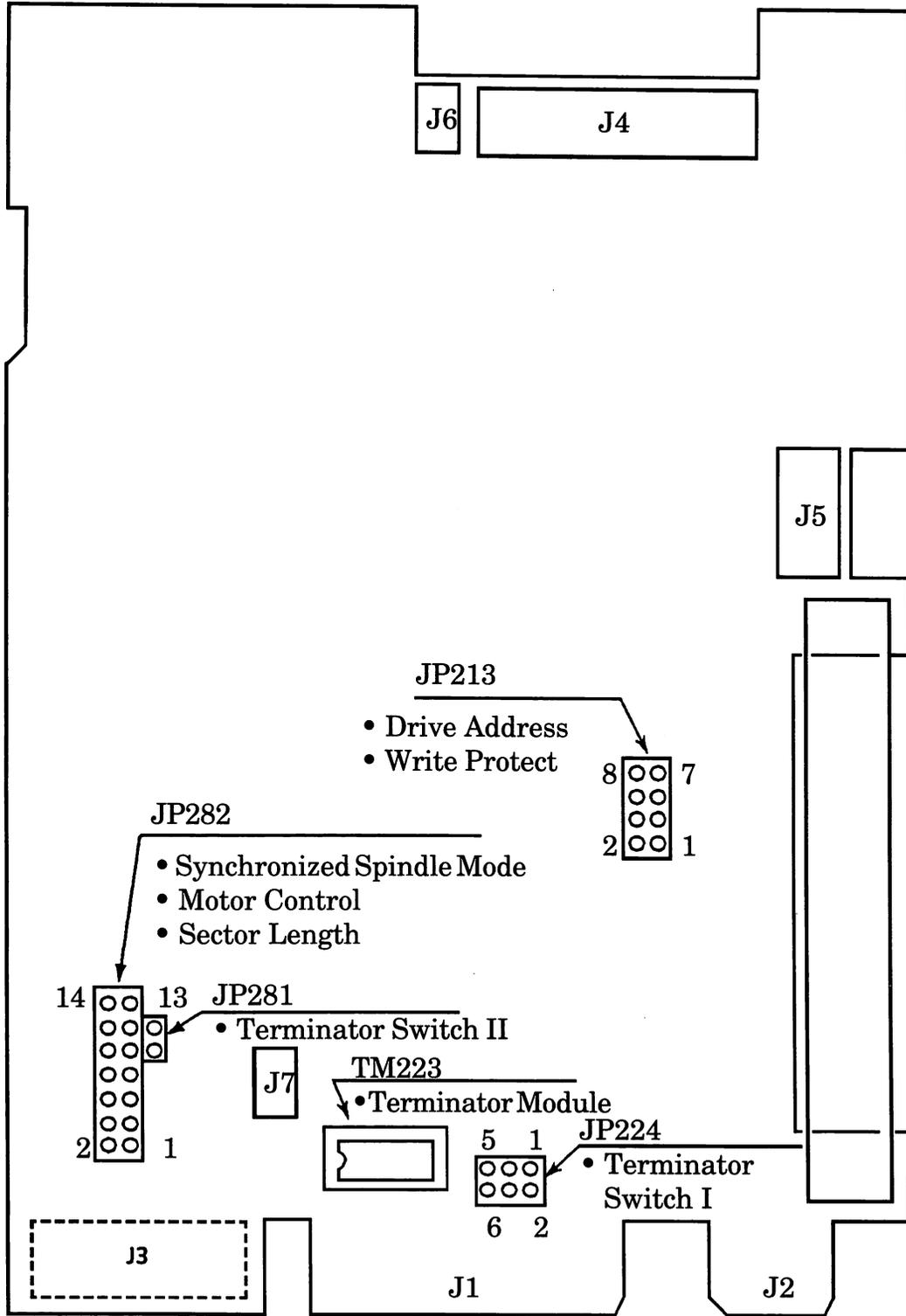
Figure 13 - SZ931 PCB Layout (PCB Rev. 0)
