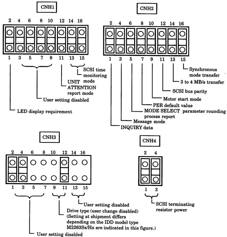
**Figure 9 – Fujitsu 226X Series Jumper Settings**
