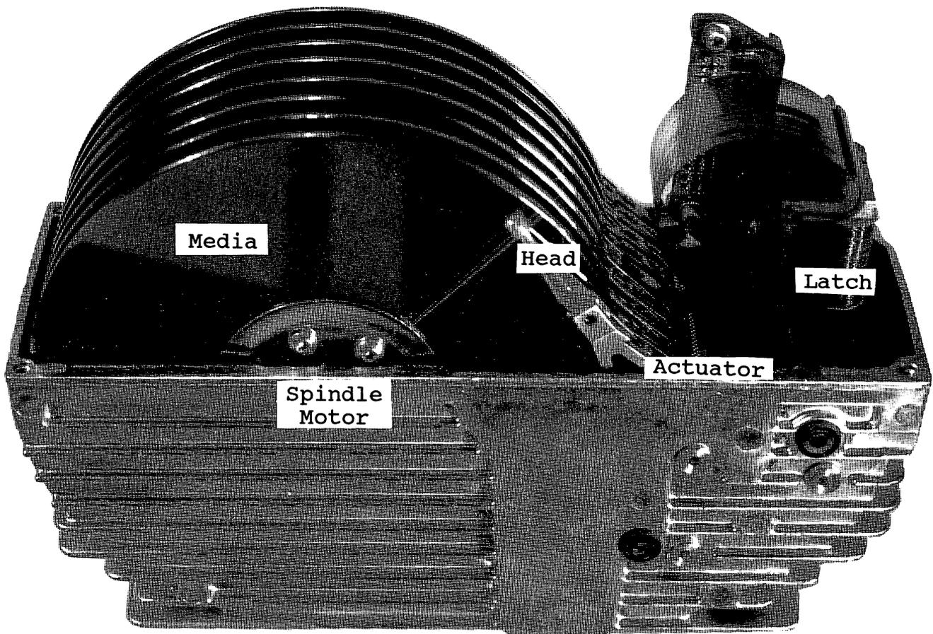
**Figure 1 - Basic Drive Operation**
