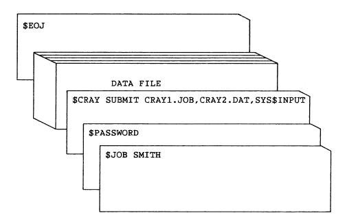
Figure 3-3. COS Job Deck for Batch Job Submission from a Card Reader
