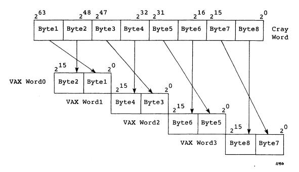
Figure 4-1. Blocked Data Reformatting
