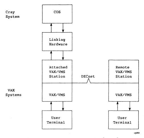
Figure 1-1. VMS/COS Hardware Configuration
