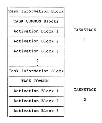
Figure F-3. Task Stacks in Managed Memory
