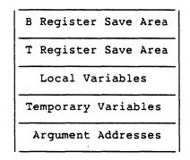
Figure F-4. Activation Block Stack Frame
