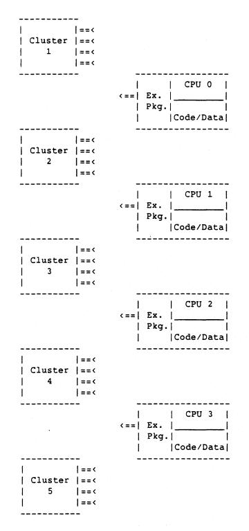
Figure 10-1. Clusters and Processors for a Four-processor CRAY X-MP Computer System
