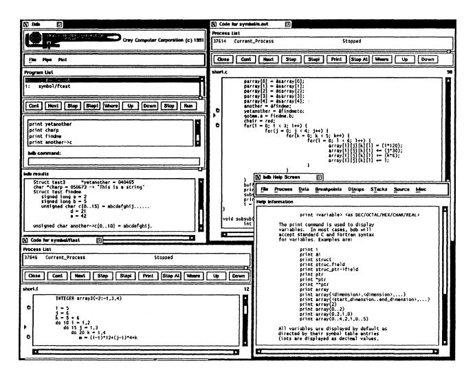
Shown in the above figure is the OSF/Motif widget version of **bdb**, which utilizes the Holmes libraries graphical user interface. Three sample screens are presented: the main screen (upper left) from which the user controls all processesses, two code windows (upper right and lower left) from which those individual processes can be controlled, and the on-line help facility (lower right).
