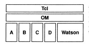
A graphical user interface has been added to the application by including Watson in the load module. With few exceptions, the control of the user interface may be completely contained in the Tcl layer as Tcl code.
