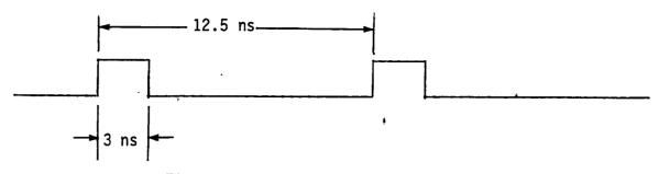
Figure 2-3. Clock pulse waveform
