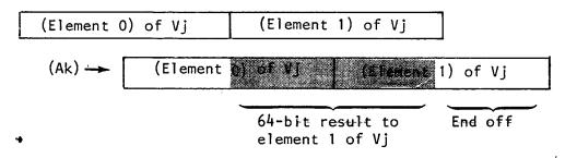
The last operation performed by the instruction joins the last element of Vj as determined by (VL) with the preceding element. The following figure illustrates this operation.
