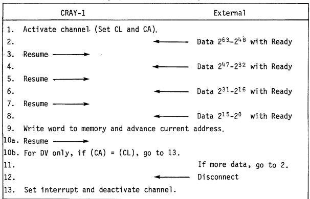
Table 6-2 16-bit asynchronous input channel signal exchange (DJ, DU, or DV modules)
