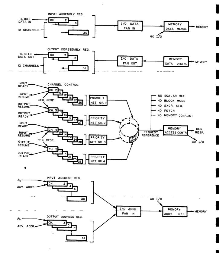
Figure 6-2. Channel I/O control
