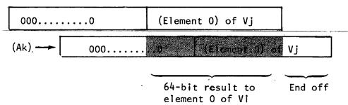
If (VL) = 1, only the one operation is performed. In the general case, however, instruction execution continues by joining element 0 with element 1, shifting the 128-bit quantity by the amount specified by (Ak), and transmitting the result to element 1 of Vi. This operation is shown below.
