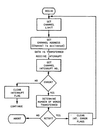
Figure 6-1. Basic I/O program flow chart
