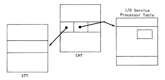
Figure 2-3. Channel table linkage
