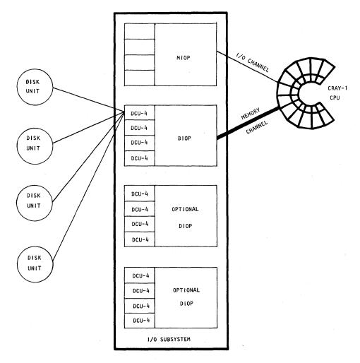
Figure 4.2-4. DCU-4 controller configuration
