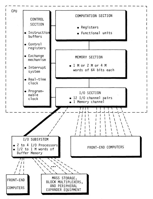
Figure 1-2. CRAY-1 S Series Model S/1200 through S/4400 Computer Systems
