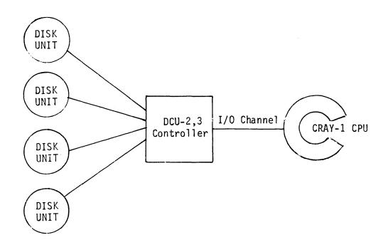
Figure 4.2-3. DCU-2, 3 Controller configuration
