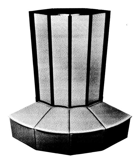
Figure 1-2. I/O Subsystem Chassis
