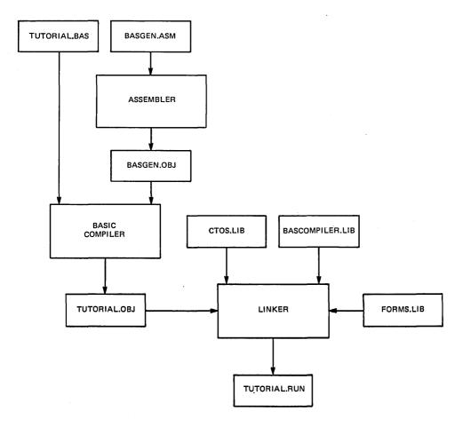
Figure B-1. Compiling and Linking a Program That calls Non-BASIC Procedures
