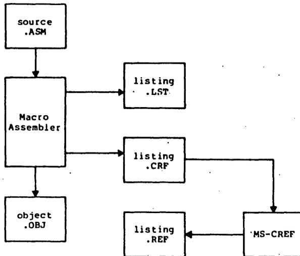
Figure 6. Files That Macro Assembler Produces
