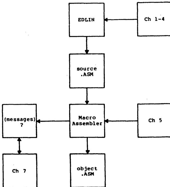
Figure 4. Overview of Macro Assembler Operation
