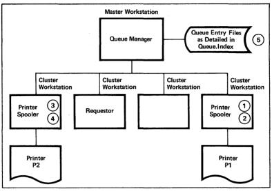
Note the corresponding entries for printer P1 and queue SPLA in Queue.Index and the Spooler Configuration File for the first printer. The Queue.Index entries for P2 and SPLB similarly correspond to entries in the Spooler Configuration File for the second printer.
