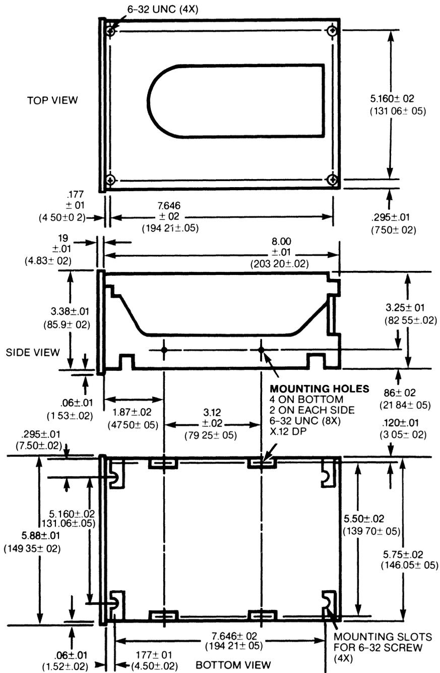
Figure 18 — MOUNTING DIMENSIONS
