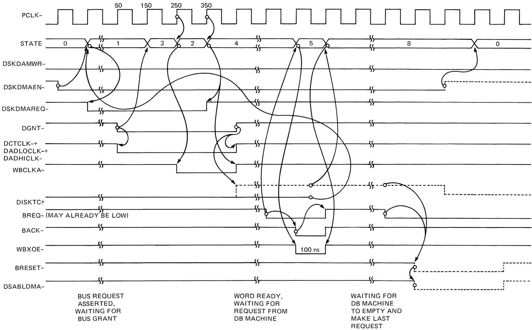
Figure 6-4. Disk Word State Machine -- Disk Write
