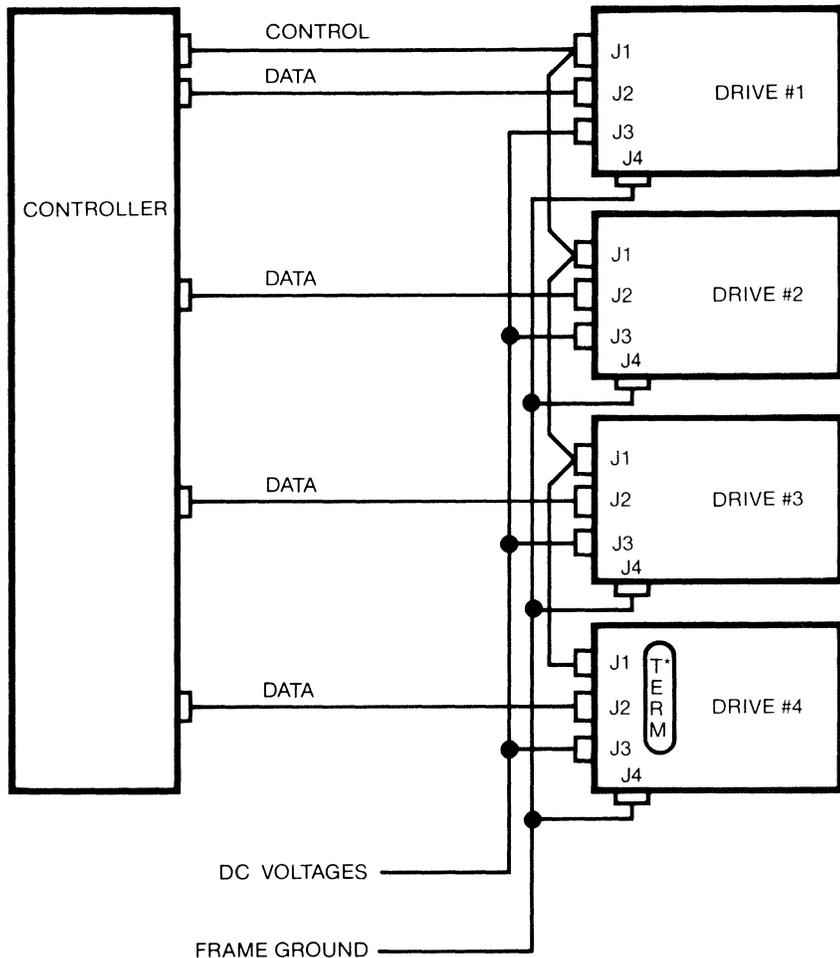
\* The last or only drive in the control cable string must have the terminator resistor pack installed. All other drives must have their terminators removed.
