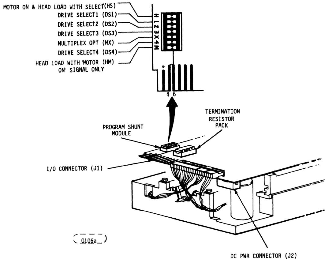
Figure 23. Program Shunt Module
