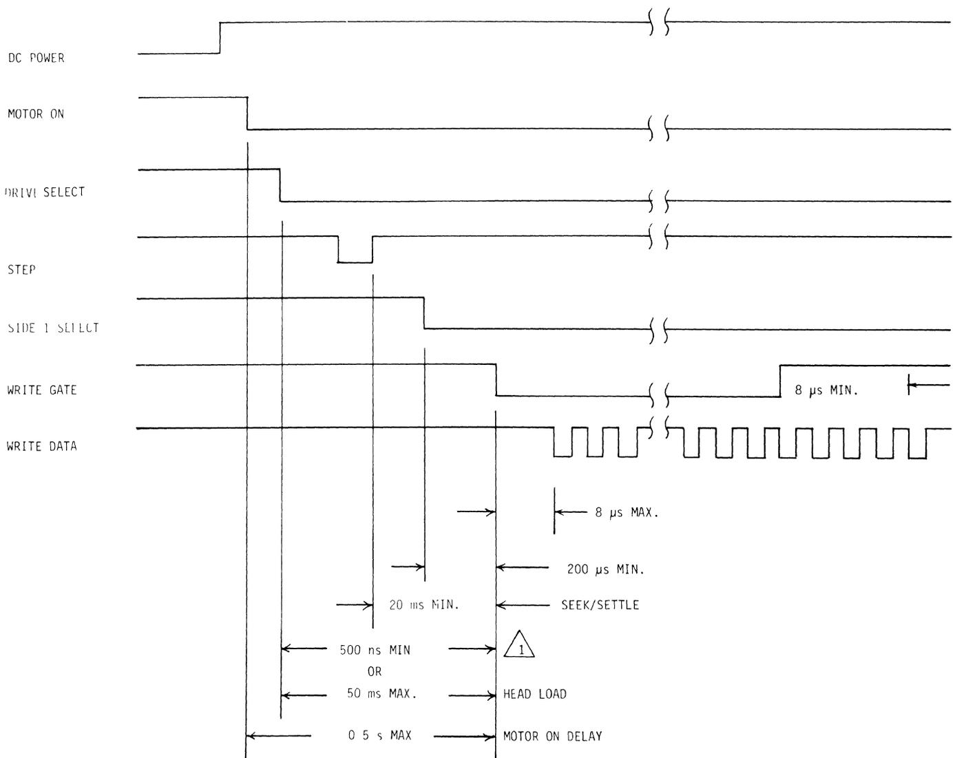
1 ASSUMES HEAD IS LOADED AND MOTOR IS UP TO SPEED WHEN DRIVE IS SELECTED.
