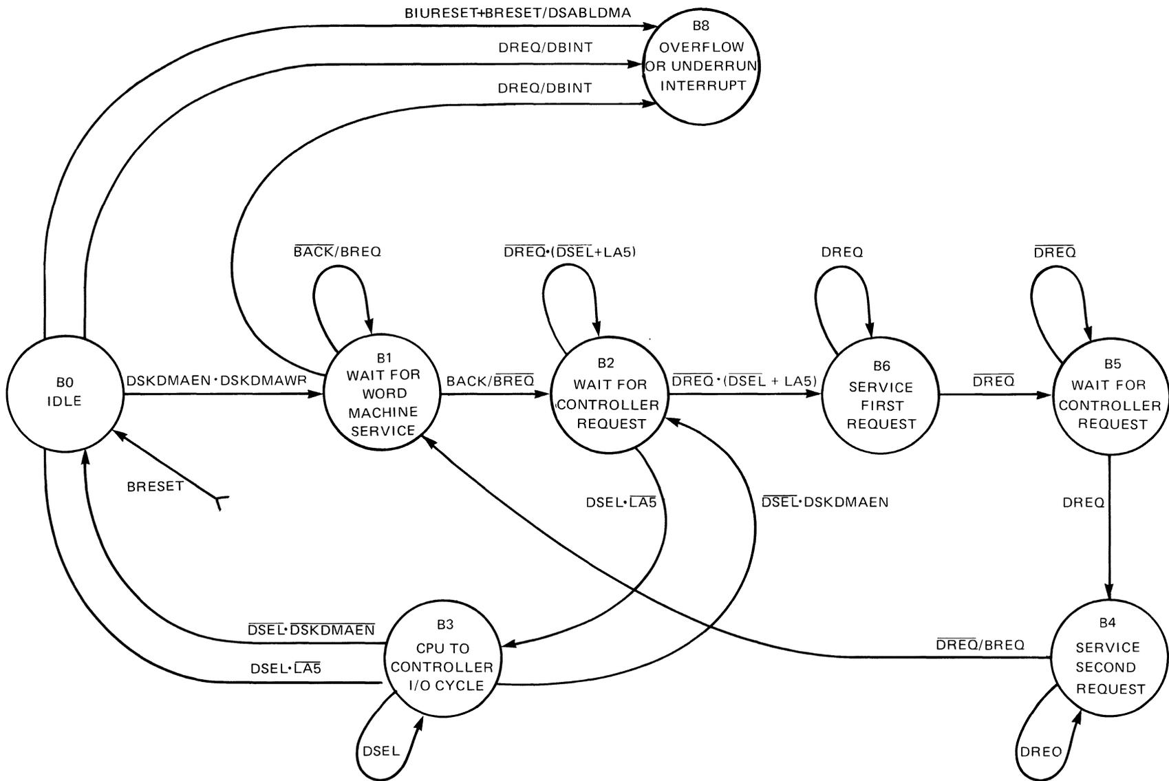
Figure 5-4. Disk Byte Machine State Sequencing Diagram
