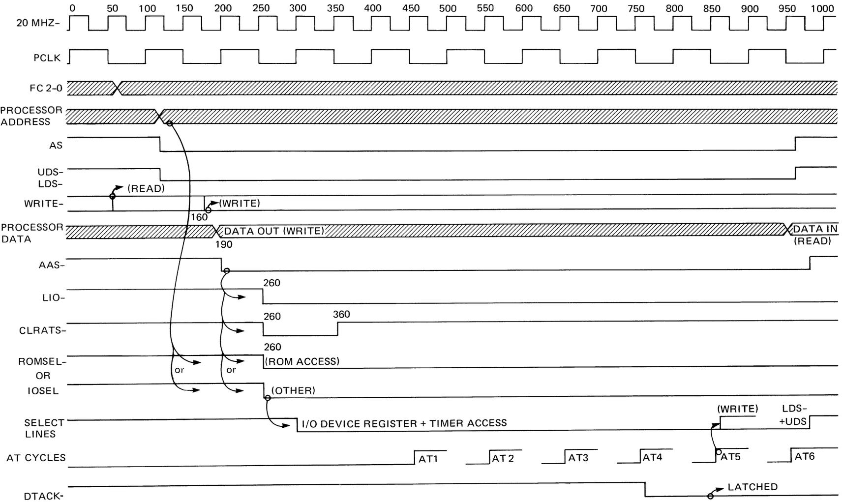
Figure 6-3. CPU Slow Cycle (Input/Output) Transfer
