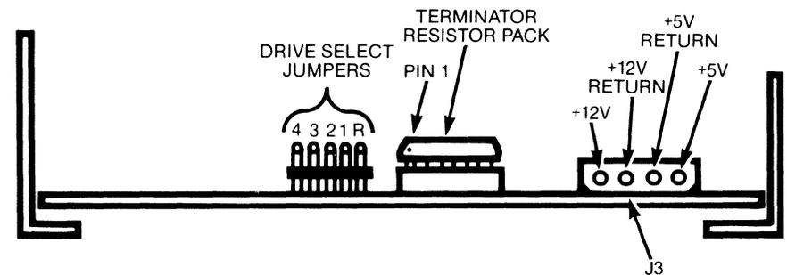
Figure 7 SELECT JUMPER, TERMINATOR AND J3 LOCATIONS
