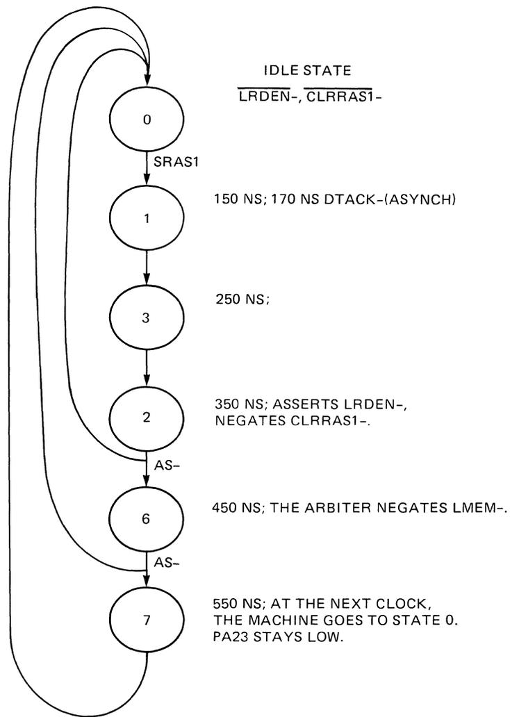
Figure 5-2. CPU State Machine State Sequencing Diagram
