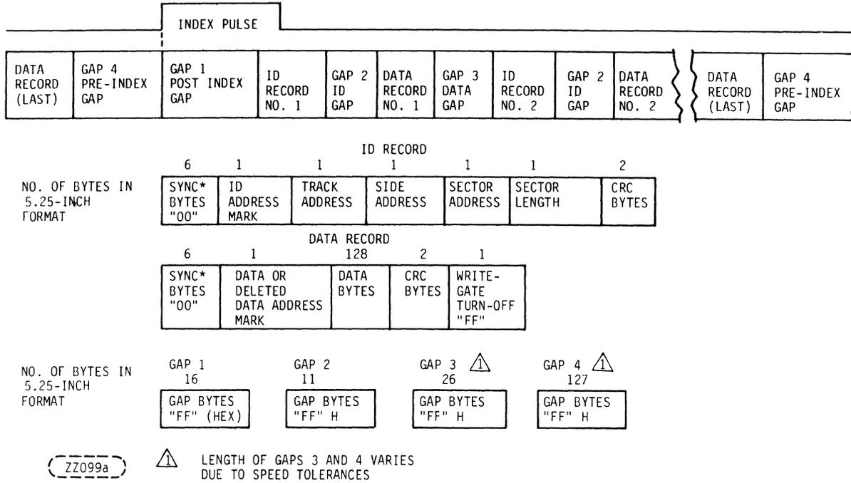
**Figure 6. Minimum Requirements for Single-Density Soft-Sector Format (Part 2)**
