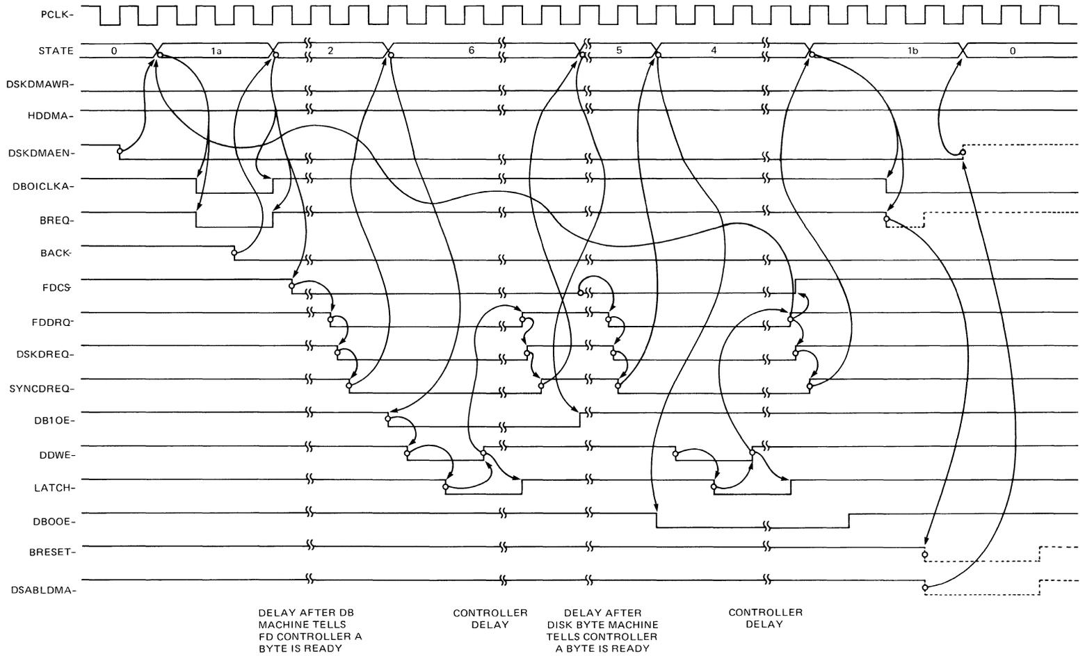
Figure 6-5. Disk Byte State Machine -- Floppy Disk Write
