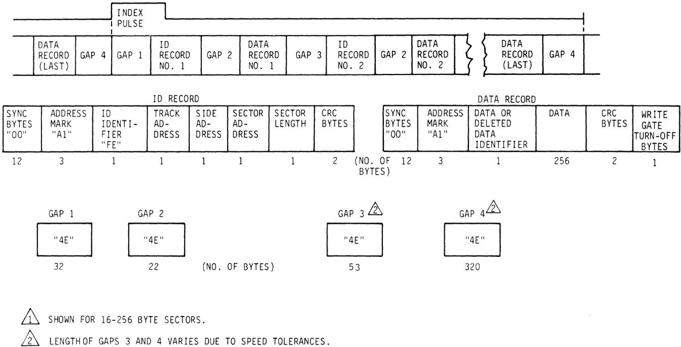
**Figure 7. Recommended Double-Density Format**
