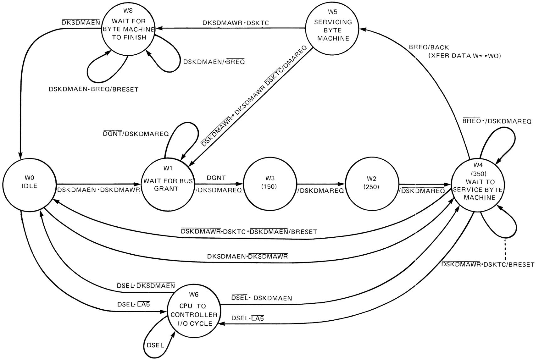
Figure 5-3. Disk Word Machine State Sequencing Diagram
