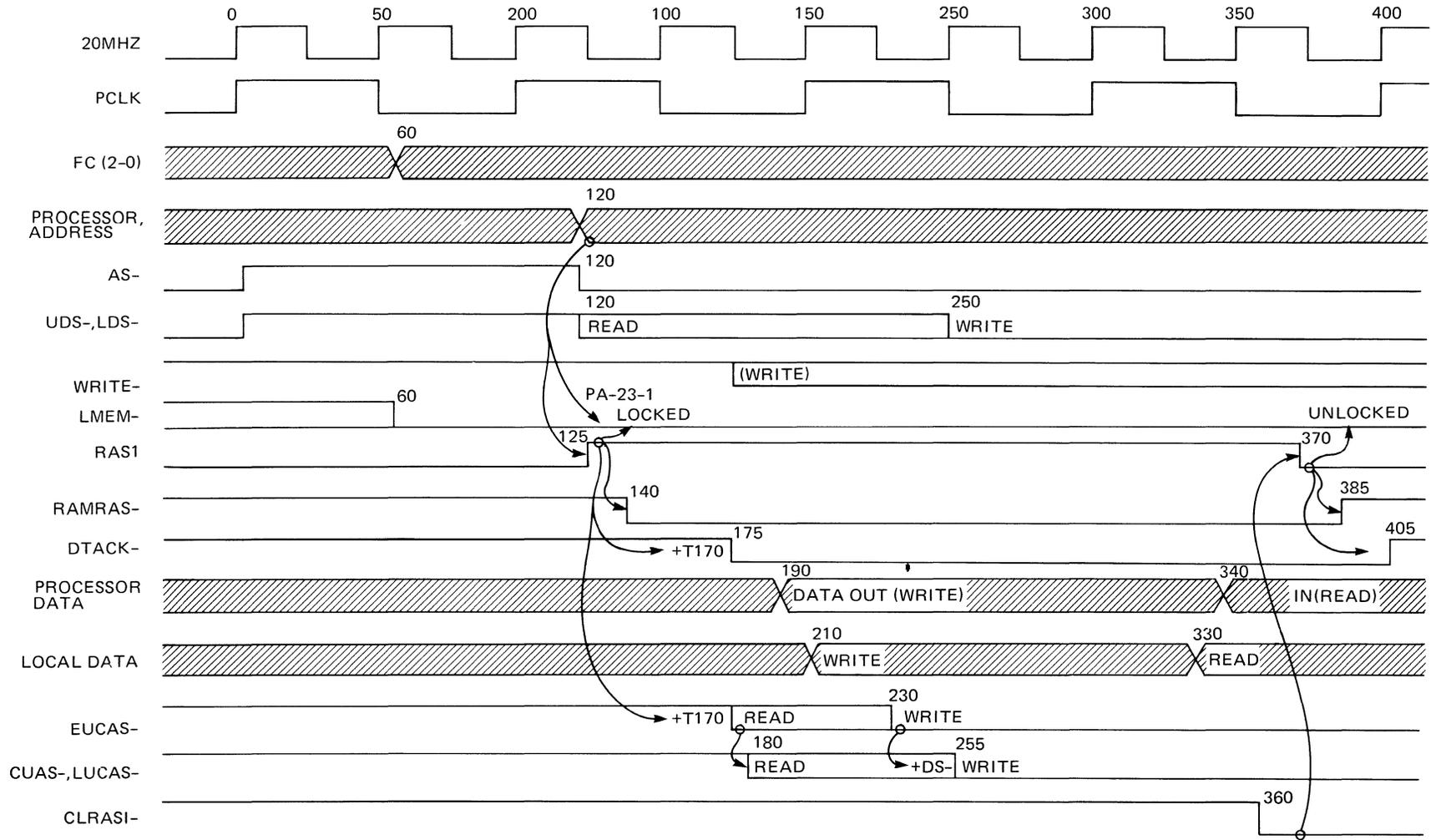
Figure 6-2. Fast Cycle Transfers -- CPU Memory Access
