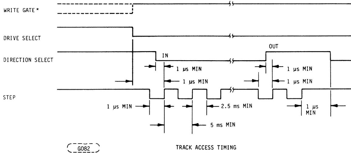
**Figure 16. Track Access Timing**
