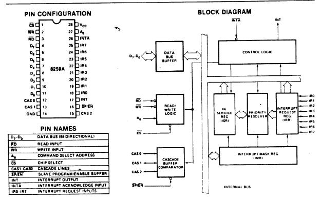
Figure 7. 8259A Block Diagram and Pin Configuration
