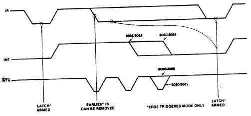
Figure 16. IR Triggering Timing Requirements
