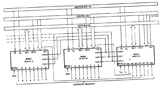
Figure 18. Cascaded 8259A'S 22 Interrupt Levels
