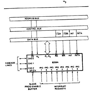
Figure 1. 8259A Interface to Standard System Bus
