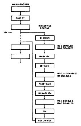
Figure 15. Special Mask Mode Example (MCS 80/85<sup>TM</sup>or MCS 86/88<sup>TM</sup>)
