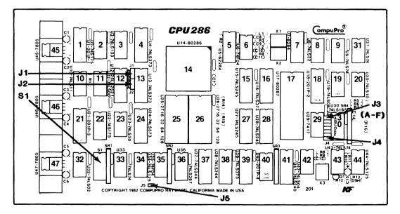
Figure 2. CPU 286 (jumper and switch location)
