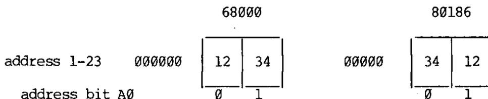
The above example shows how the 2 CPU chips store the hexadecimal word '1234' in memory. The swap built into the VME-80186 allows all data interchange between CPU's to be programmer transparent. The 80186 programmer should not write words on odd memory addresses if the 68000 is to correctly read this data, since the 68000 chip itself cannot support this feature.
